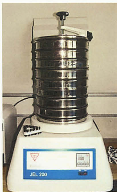
Figure 2: A mechanical shaker used for sieve analysis.
