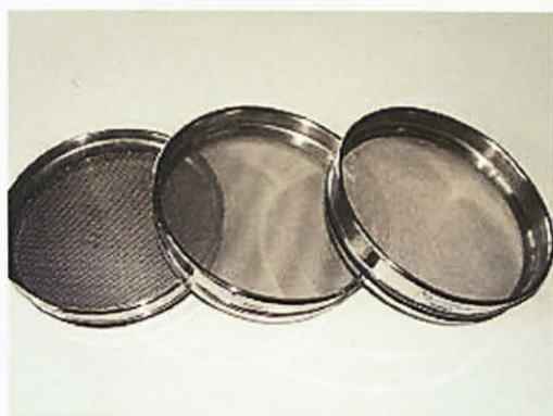
Figure 1: Sieves used for gradation test.
