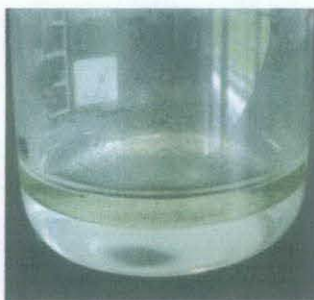
Figure 4.1: Two phase systems after left for 18 hours
