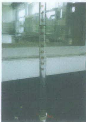
Figure 4.2: Titration method is used to separate top and bottom phase
