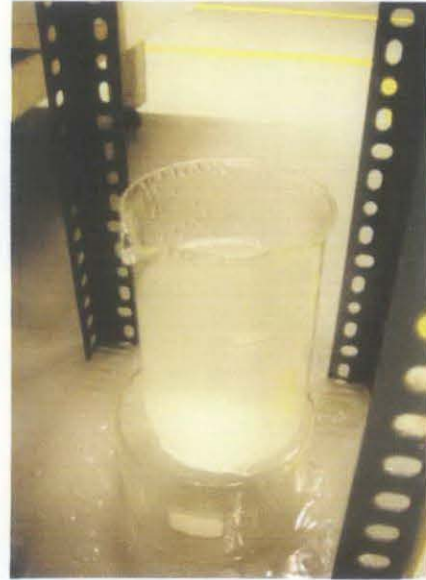
Figure 4.5: Filtrate turbidity after treating 6% oil + water mixture with 0.02 \text{ g/cm}^3 Kapok filter
