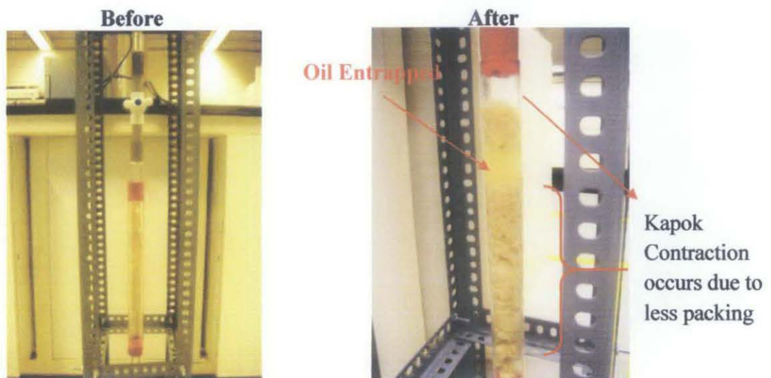
Figure 4.3: 0.02 g/cm 3 Kapok Filter before and after treating 6% oil + water mixture
