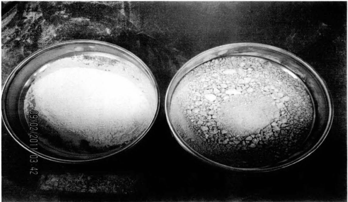
Figure 5: Limestone powder form 63 micron, and small grains
