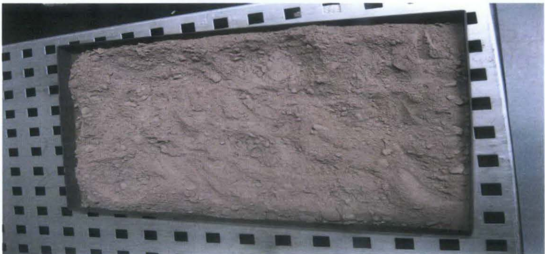
Figure 10: A mixture of raw materials ready for clinkering
