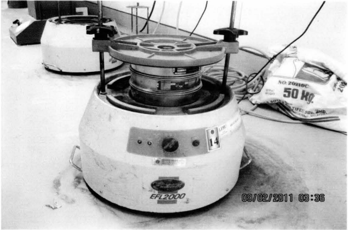
Figure 4: SIVE Shaker, Civil Engineering, Block13
