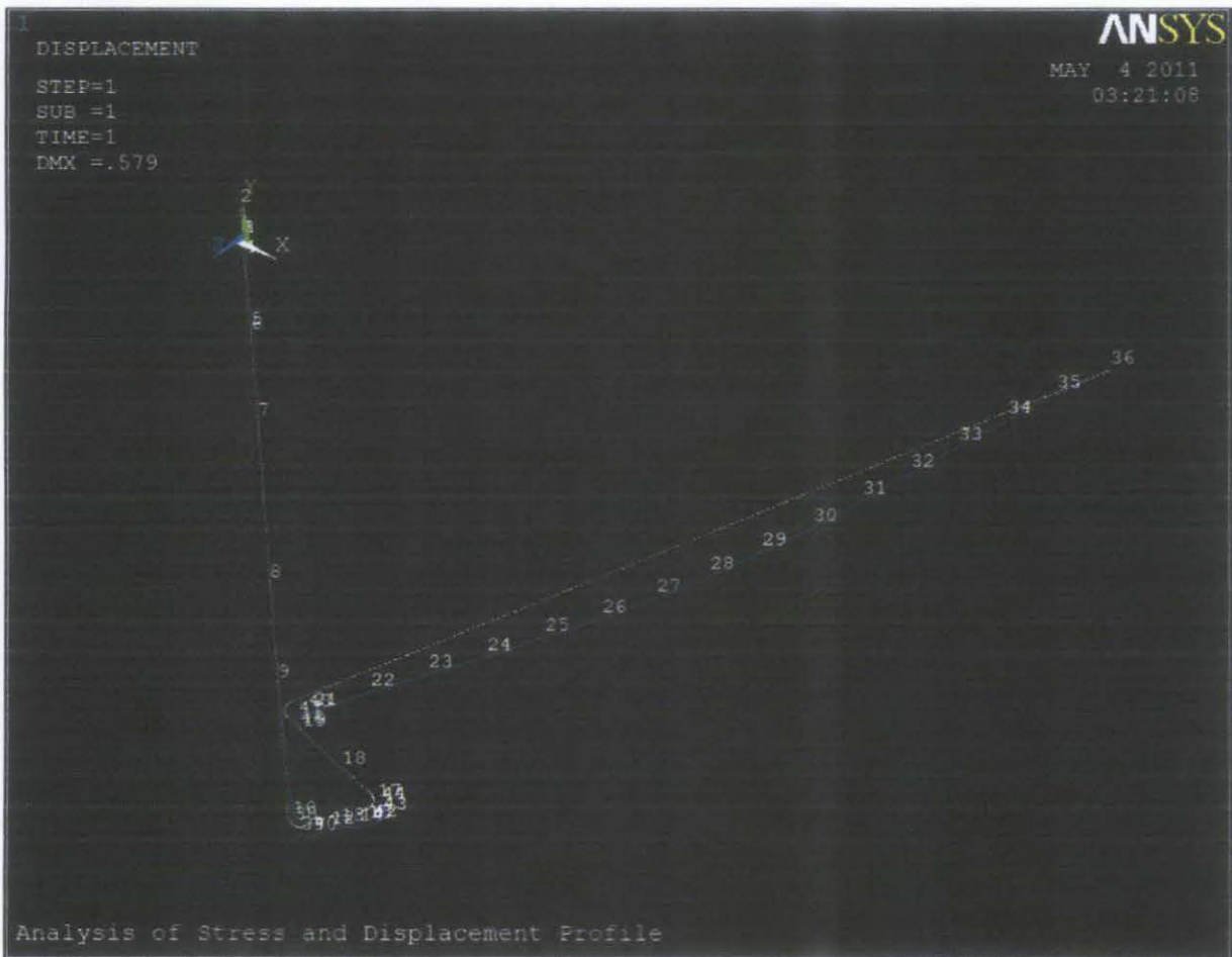
Figure 4.3 : Original and Deformed Pipeline after Simulation
