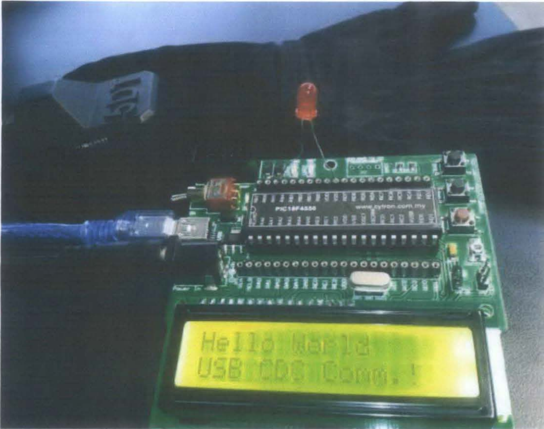
Figure 43: Interfacing the PIC and Data Glove (note all LED indicators are OFF)
