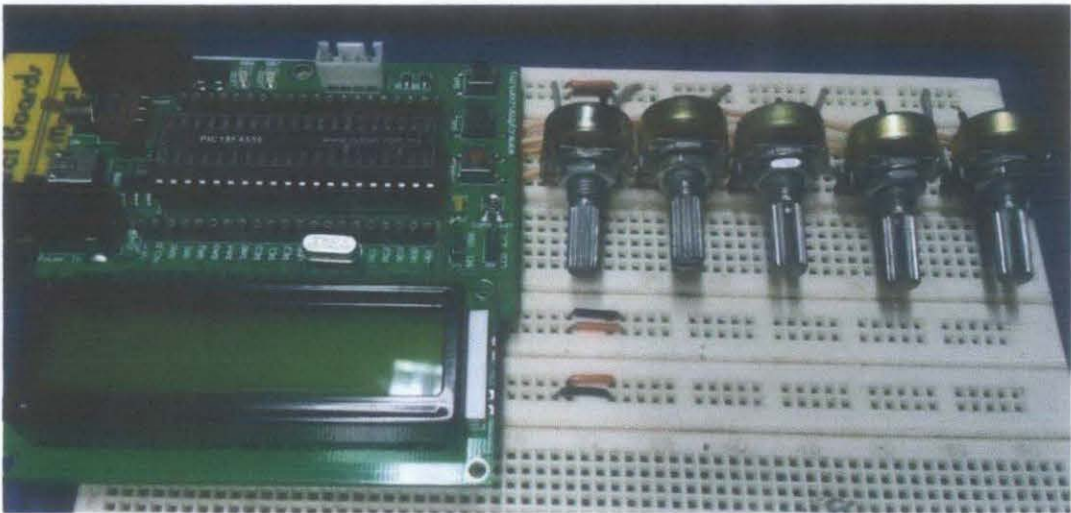
Figure 21: Translation System Components: 5 Potentiometers, Main Board (SK40C board), and LCD
