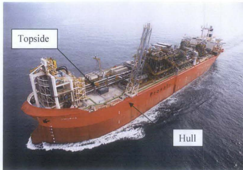
Figure 5: Hull Section and Topside of FPSO [20]
