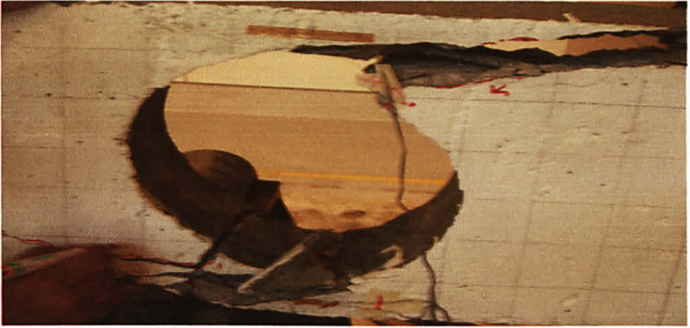
Figure 4.12: Failure of beam with large circular opening at support. Please refer appendix 6 for the load versus deflection results for static load test.
