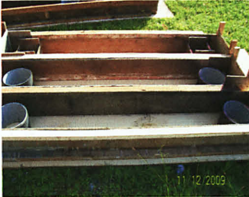
Figure3.4: Special opening created at critical shear zone with \Phi 230\text{mm} for the circular opening and 210\text{mm} \times 210\text{mm} for the square opening. The square opening was made using the spare wood and the circular opening was prepared using PVC pipes cut to the required size and depth. As the exact size of opening of the PVC pipe was not available at the market, the PVC size slightly smaller was glued with a rubber sheet with thickness sufficient to add the lack of opening size of the PVC to make \Phi 230\text{mm} .
