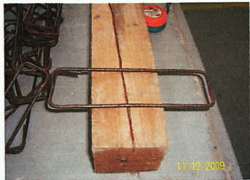
Figure 3.5: Bending of R6 links ( \Phi 6\text{mm} ) with dimension 3'' \times 11'' or 76\text{mm} \times 280\text{mm} .
