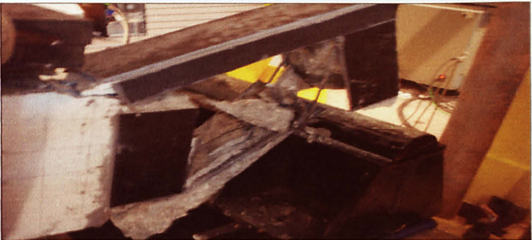
Figure 4.15: Failure of beam with large square opening at support (CFRP Strengthened)
