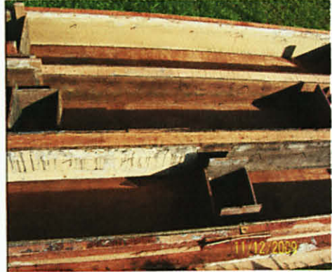
Figure3.4: Special opening created at critical shear zone with \Phi 230\text{mm} for the circular opening and 210\text{mm} \times 210\text{mm} for the square opening. The square opening was made using the spare wood and the circular opening was prepared using PVC pipes cut to the required size and depth. As the exact size of opening of the PVC pipe was not available at the market, the PVC size slightly smaller was glued with a rubber sheet with thickness sufficient to add the lack of opening size of the PVC to make \Phi 230\text{mm} .
