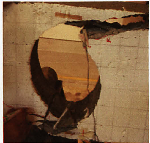
Figure 4.12: Failure of beam with large circular opening at support. Please refer appendix 6 for the load versus deflection results for static load test.
