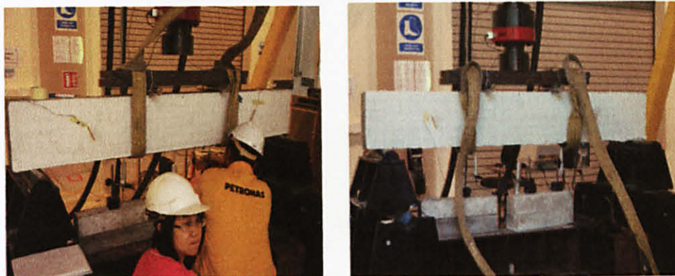
Figure4.6: Preparation for static load for control beam using the self straining Loading frame attached to a dynamic actuator (500kN) simply supported.
