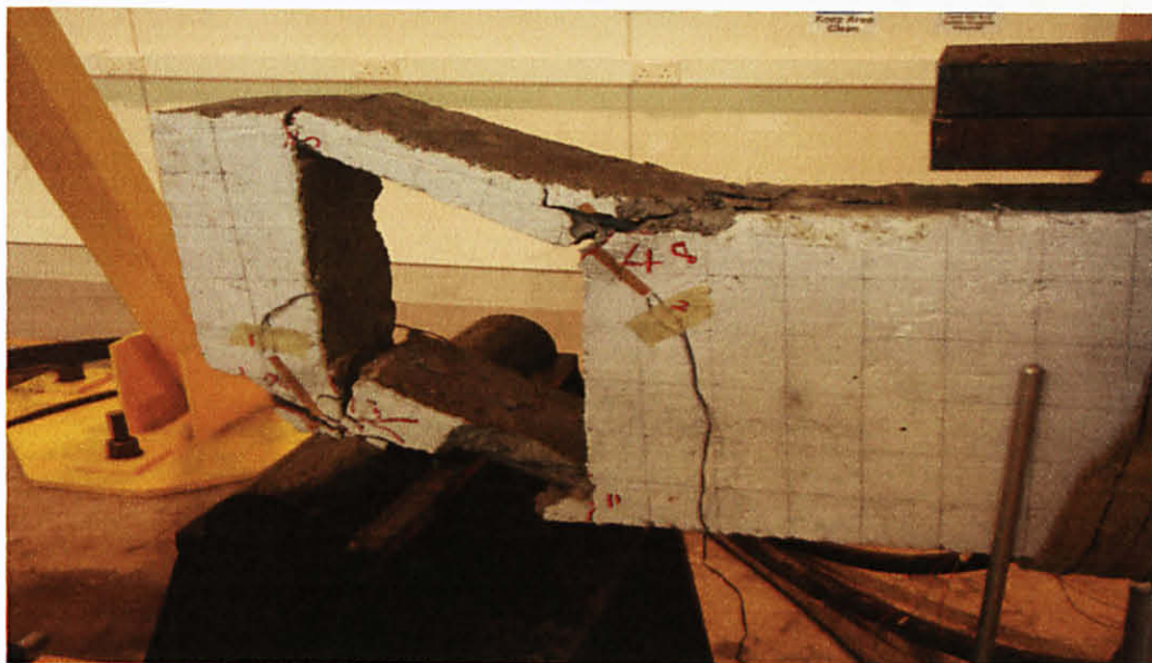
Figure 4.10: Failure of beam with large square opening at support.
