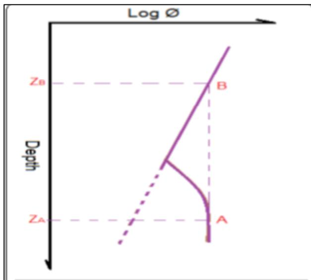
Figure 9 Porosity vs. Depth <sup>[11]</sup>
