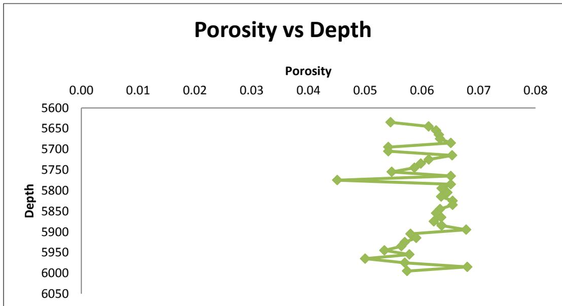
Figure 26 Porosity vs Depth Barnett Shale Well A
