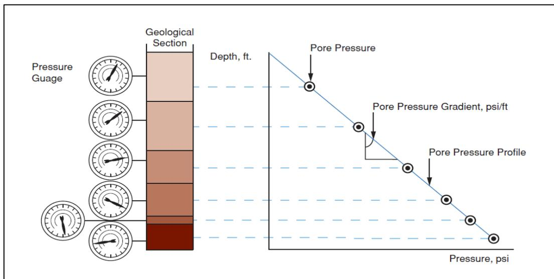
**Figure 6 P-Z Diagram Representing Pore Pressure**<sup>[8]</sup>
