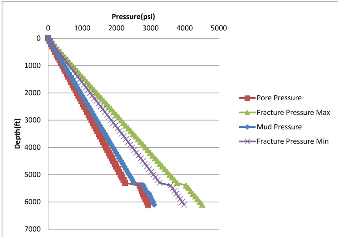
**Figure 16 Pressure vs Depth Barnett Shale Well B**
