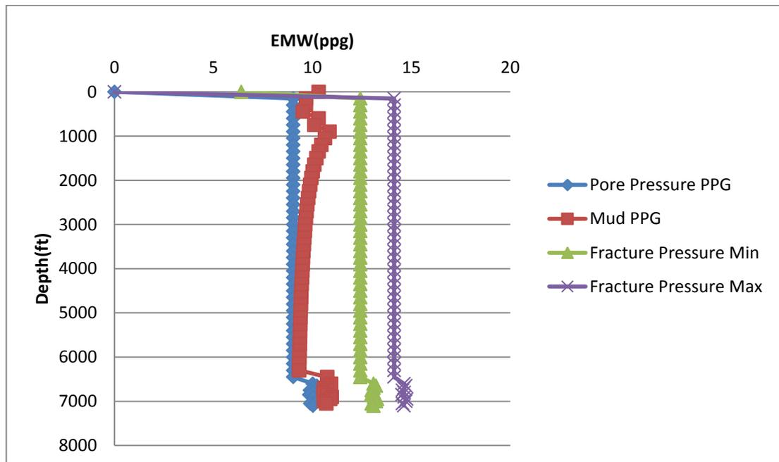
**Figure 20 EMW vs Depth Marcellus Shale Well A**
