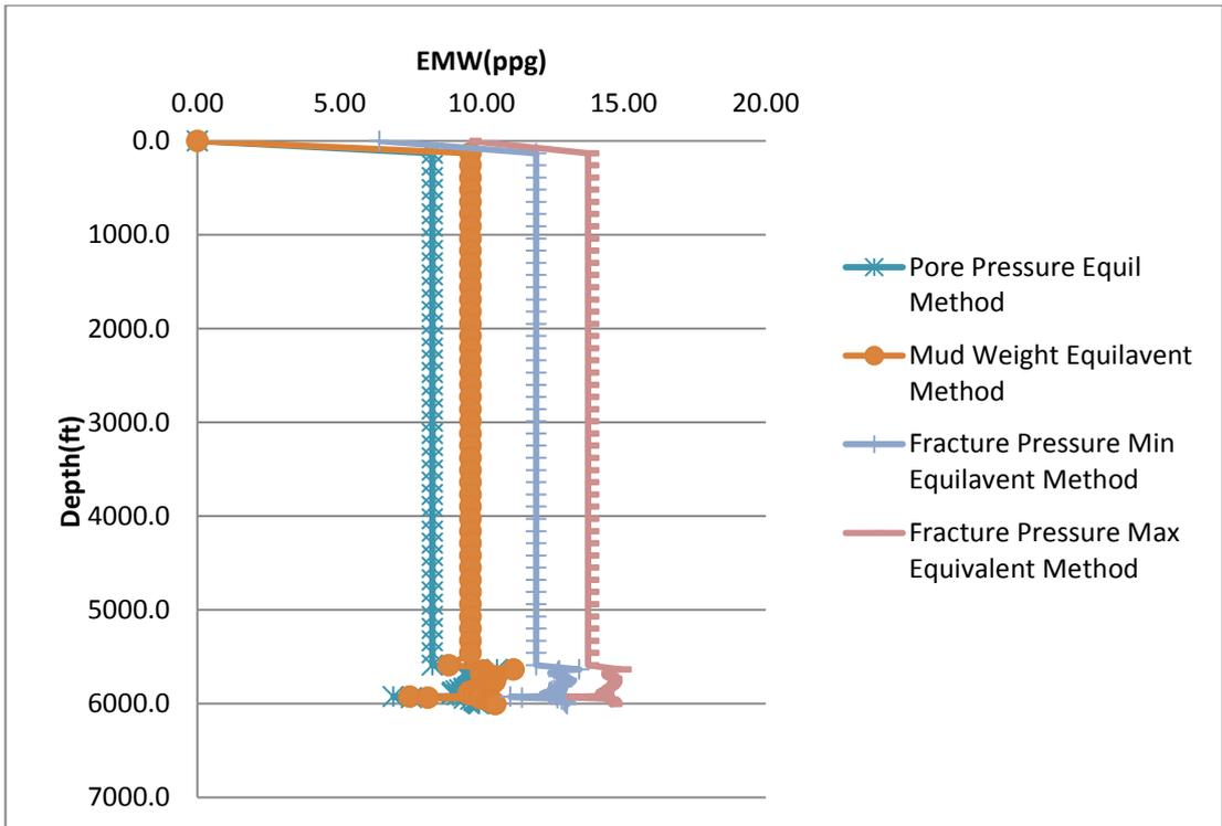
Figure 13 EMW vs Depth Barnett Shale Well A (Equivalent Method)
