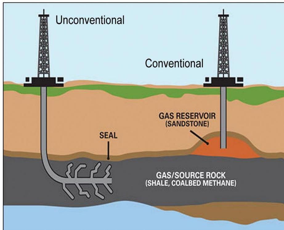
**Figure 2 Conventional vs. Unconventional Gas Production <sup>[4]</sup>**
