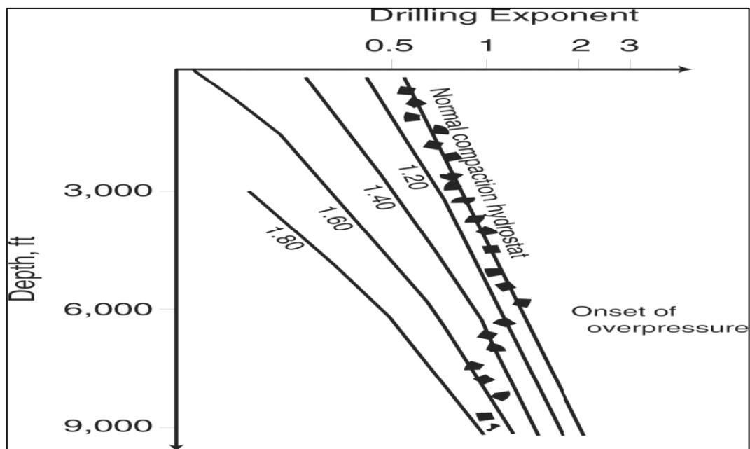
Figure 8 Drilling Exponent vs Depth<sup>[10]</sup>
