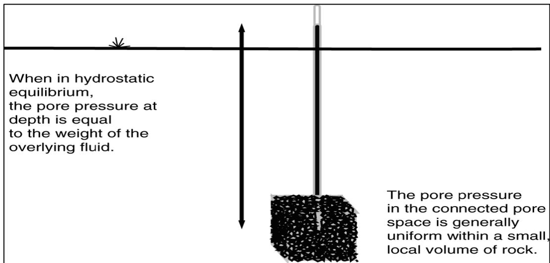
Figure 5 Illustration of pore pressure in permeable rock under hydrostatic pressure<sup>[7]</sup>
