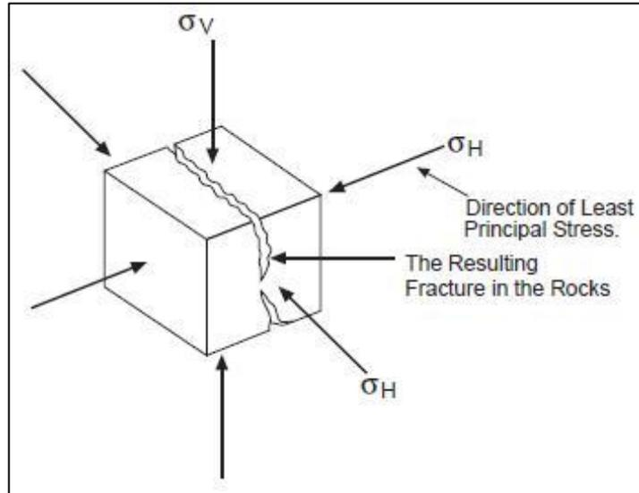
Figure 10 Fracture Pressure Stresses<sup>[18]</sup>
