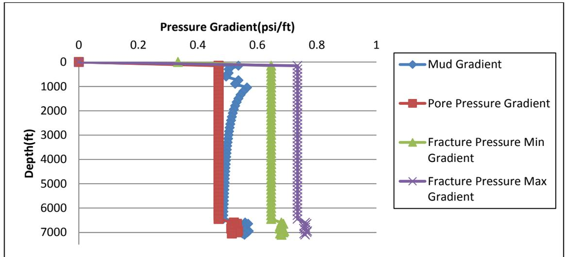
Figure 18 Pressure Gradient vs Depth Marcellus Shale Well A
