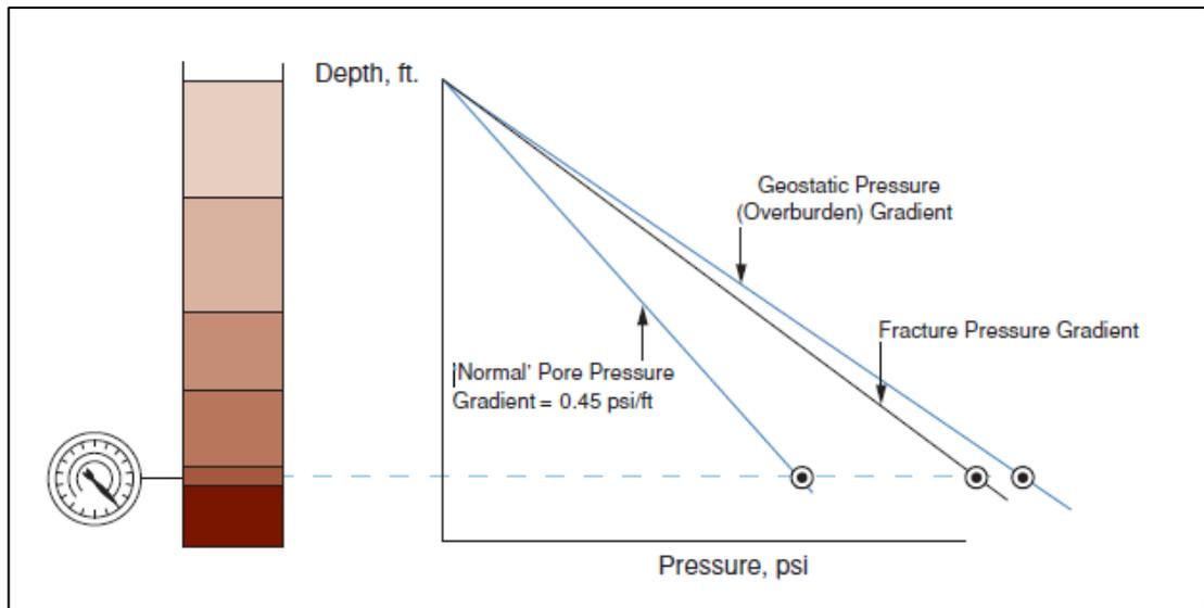
**Figure 7 Pore Pressure, Fracture Pressure and Overburden Pressures and Gradients<sup>[8]</sup>**
