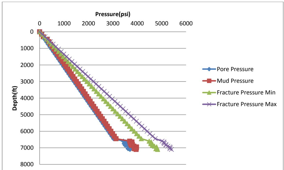
Figure 19 Pressure vs Depth Marcellus Shale Well A
