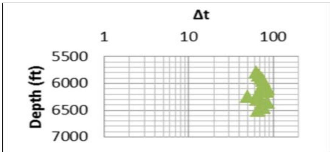
Figure 30 Sonic Velocity vs. Depth Marcellus Shale Well B
