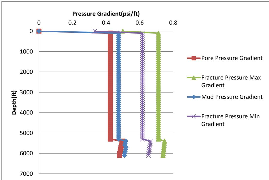
Figure 15 Pressure Gradient vs Depth Barnett Shale Well B
