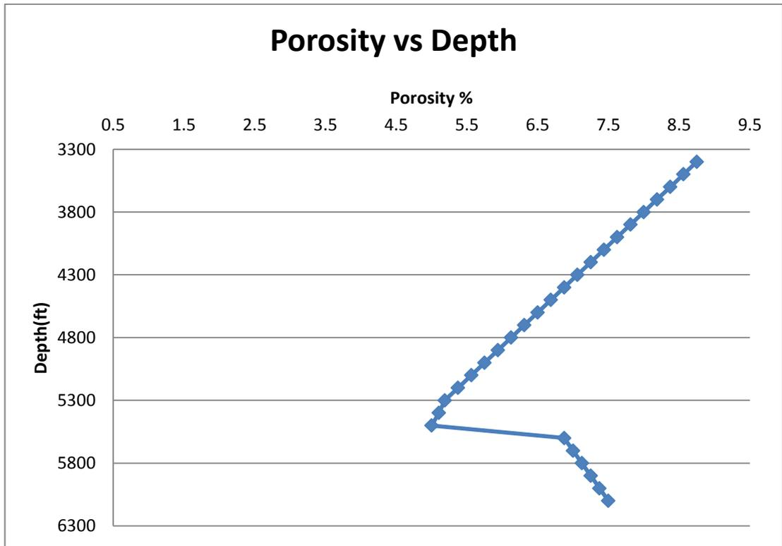
Figure 27 Porosity vs Depth Barnett Shale Well B
