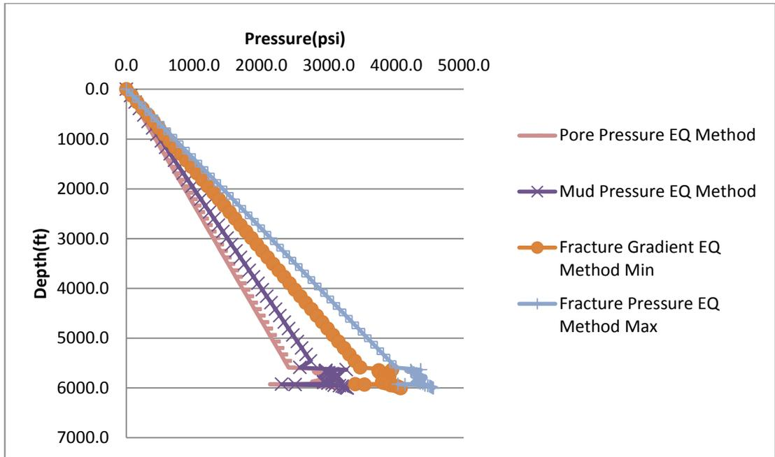
Figure 11 Pressure vs Depth Barnett Shale Well A (Equivalent Method)
