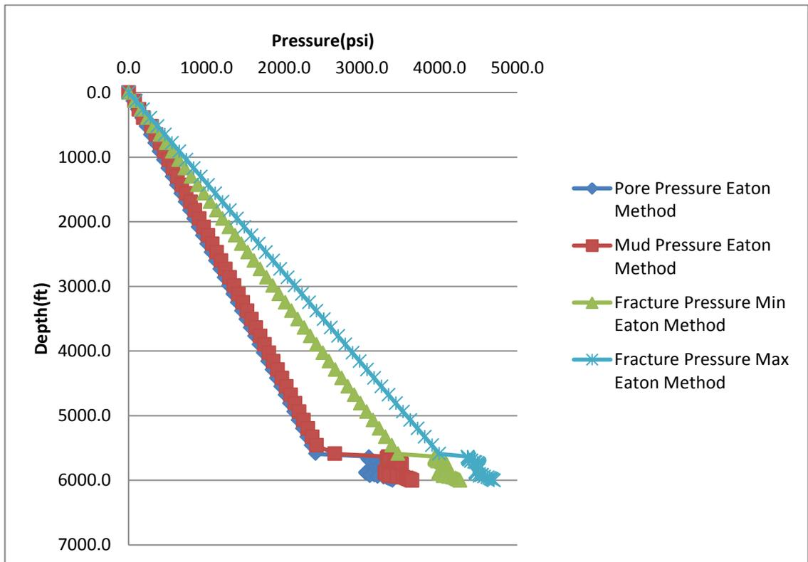
Figure 12 Pressure vs Depth Barnett Shale Well A (Eaton Method)
