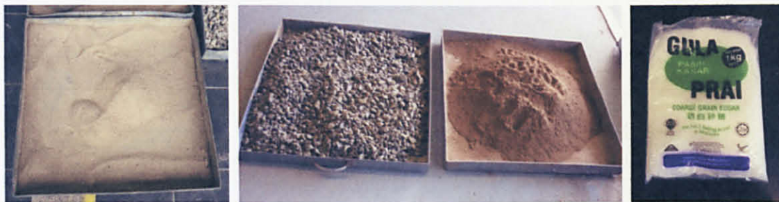
Figure 3.1 : Fine, Coarse aggregates, Fly ash and Sucrose
