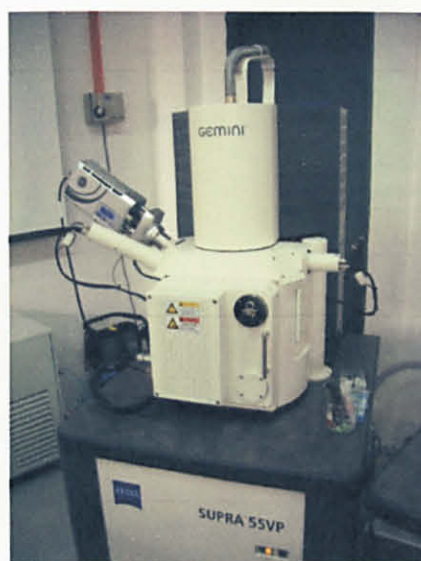
Figure 3.11: Supra 55 VP Inca X-Act Oxford FESEM Instrument
