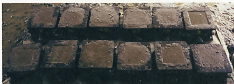
Figure 3.3 : 100 x 100 x 100 mm Steel Cube Mould
