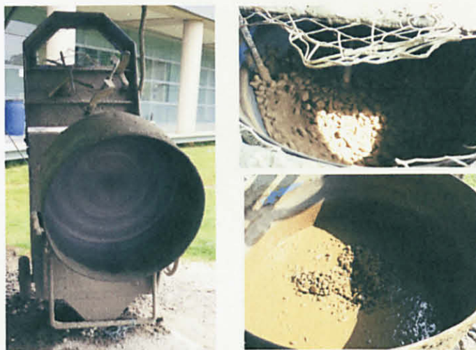
Figure 3.2 : Rotating Pan Mixer and Fresh Geopolymer Concrete
