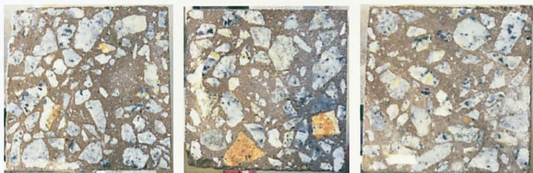
Figure 4.10: Inner Structure of Geopolymer Concrete Cured in (a) Ambient, (b) External Exposure, and (c) Oven Curing
