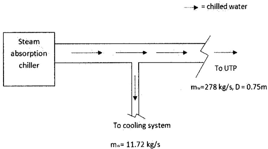
Figure 10: distribution of chilled water mass flowrate
