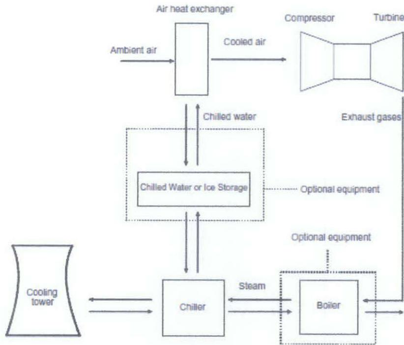
Figure 4: Generic inlet air cooling system [10]
