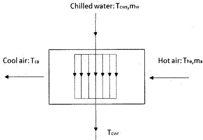
Figure 9: System diagram
