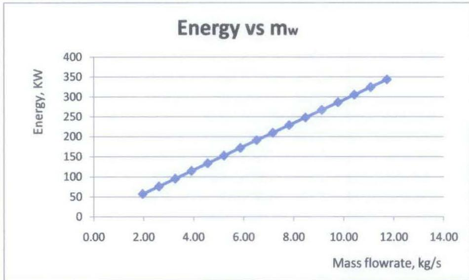
Figure 15: Energy versus water mass flowrate
