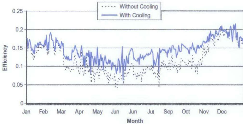
Figure 2: Average daily turbine thermal efficiency [8]
