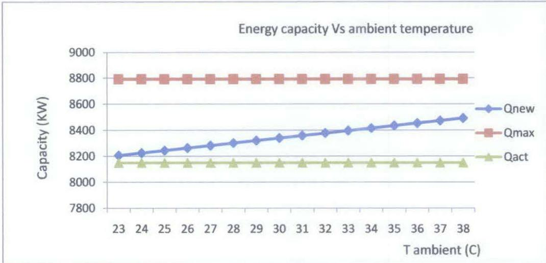
Figure 14: Energy capacity versus ambient temperature
