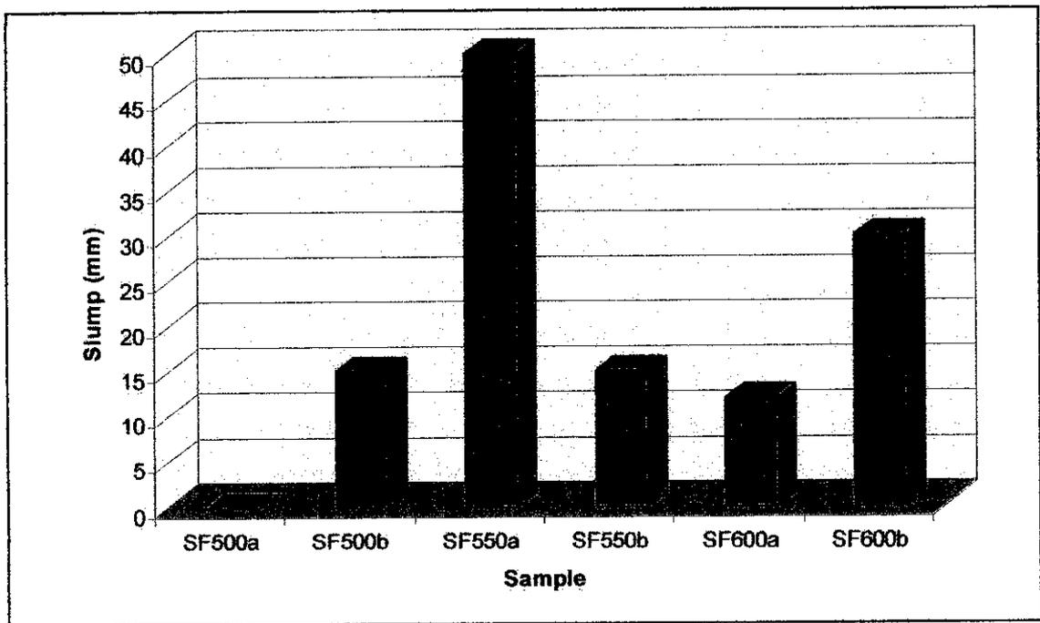
**Figure 4.1: Slump for each sample of concrete mixes**
