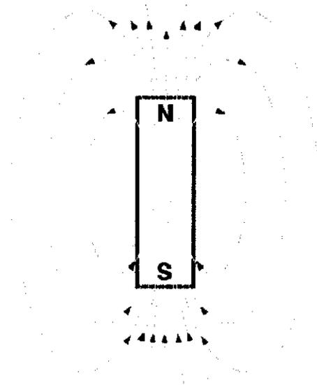
Figure 2.1: Magnetic Field Lines
