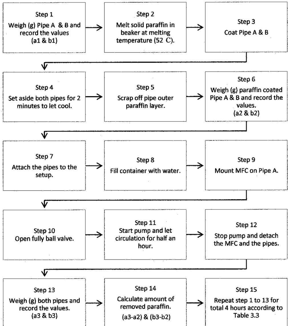
Figure 3.3: Experiment procedure
