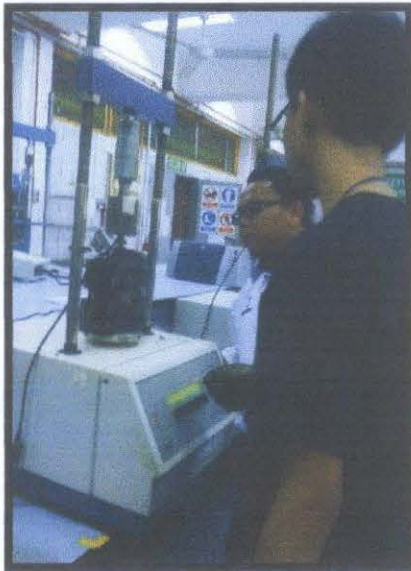
Figure 2: Obtaining the result for Marshall Test
