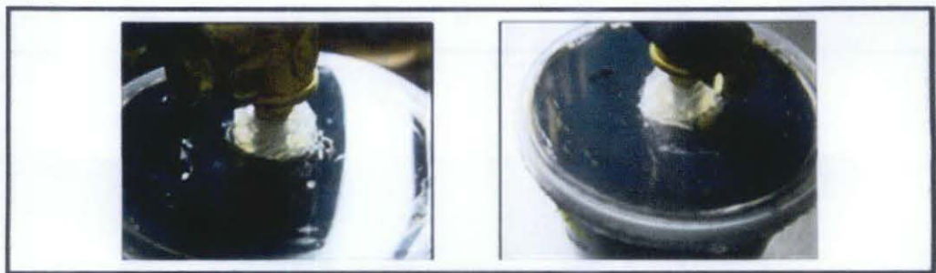
Figure 14: Gas voids formation
