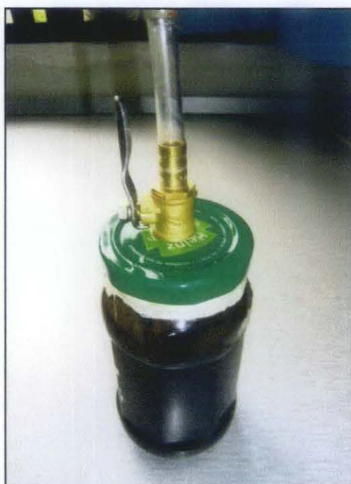
Figure 23: High pressure resistant crude tank
