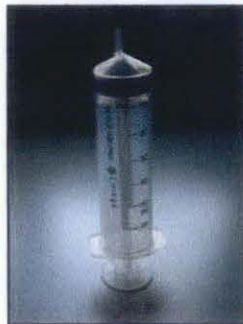
Figure 16: Syringe for gas voids storage
