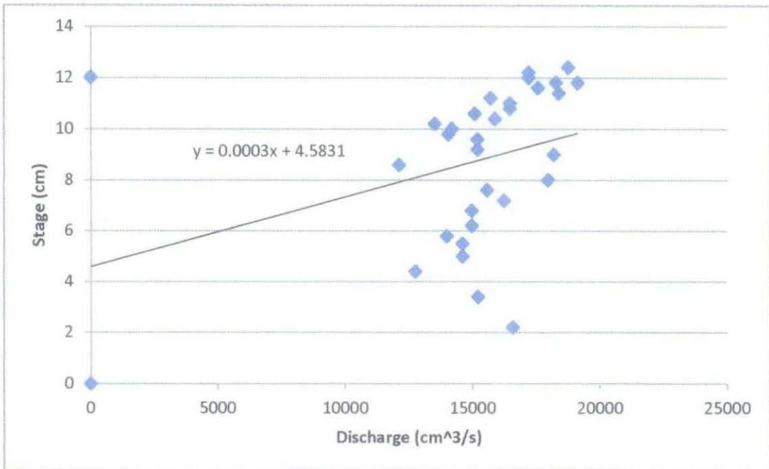
Figure 4.12: Stage versus discharge for rotation three
