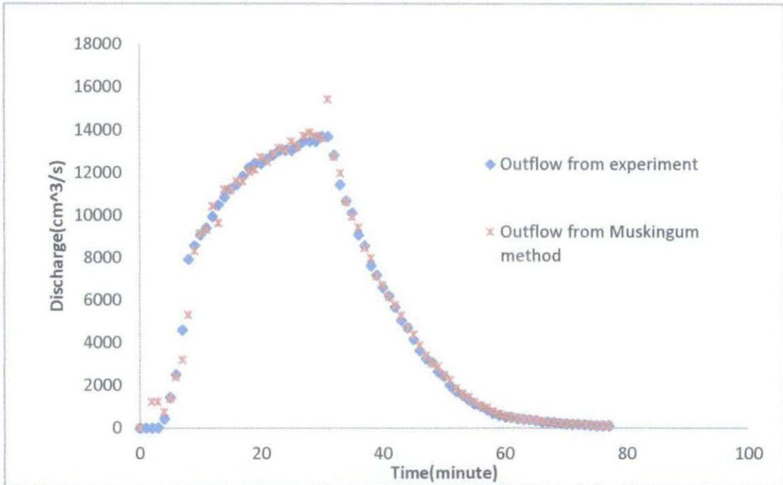
Figure 4.9: Comparison of theoretical and experimental outflow for rotation three
