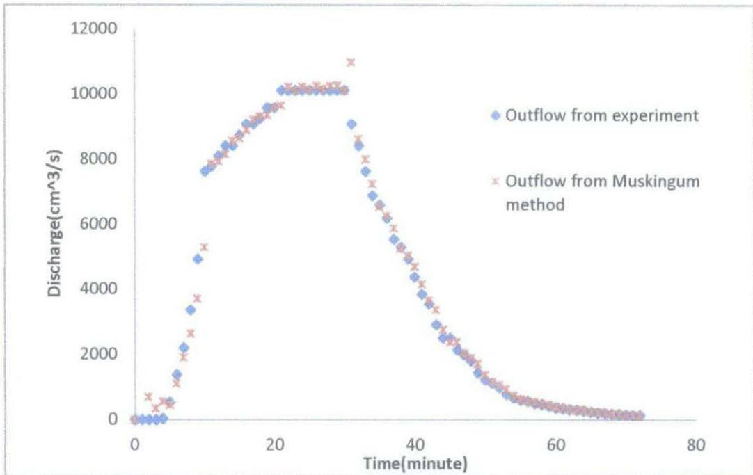
Figure 4.8: Comparison of theoretical and experimental outflow for rotation two
