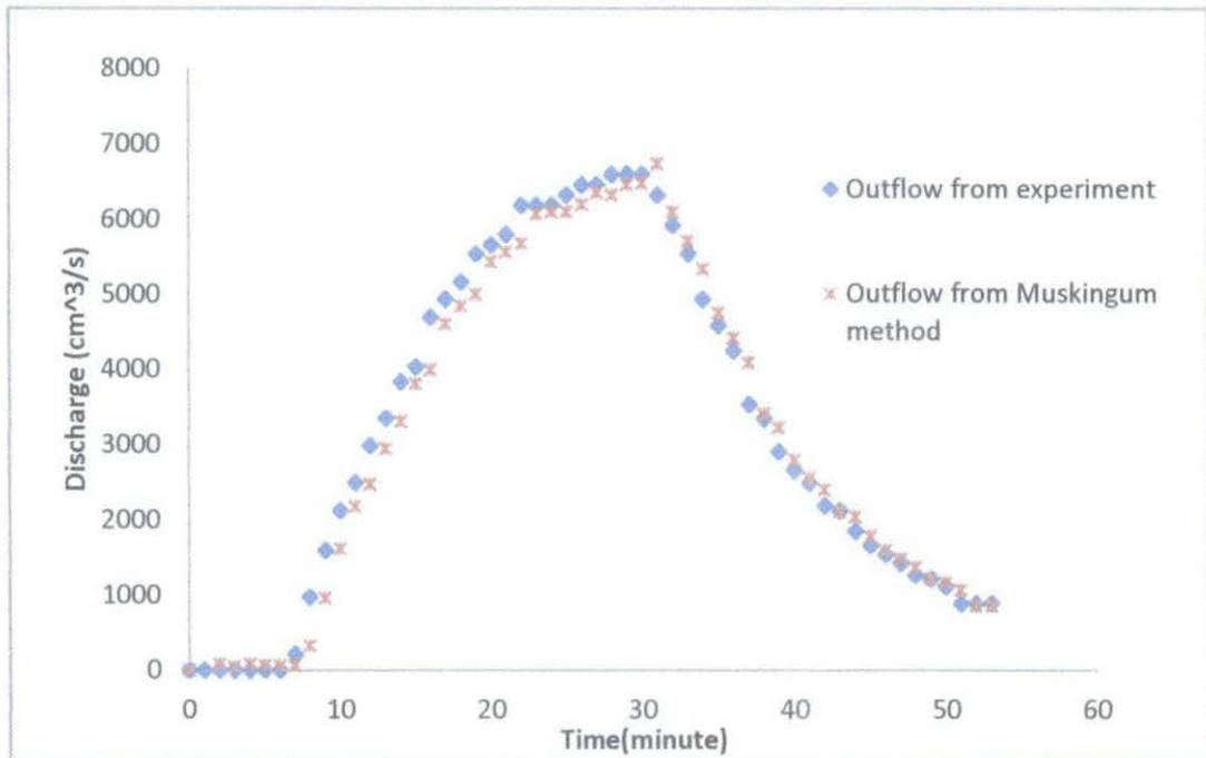
Figure 4.7: Comparison of theoretical and experimental outflow for rotation one
