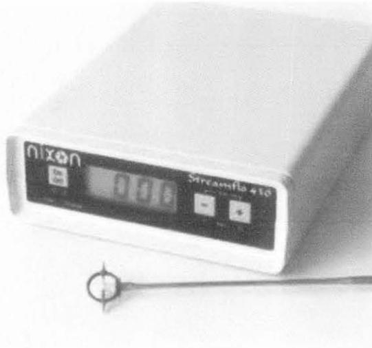
Figure 3.8: Streamflo probe
