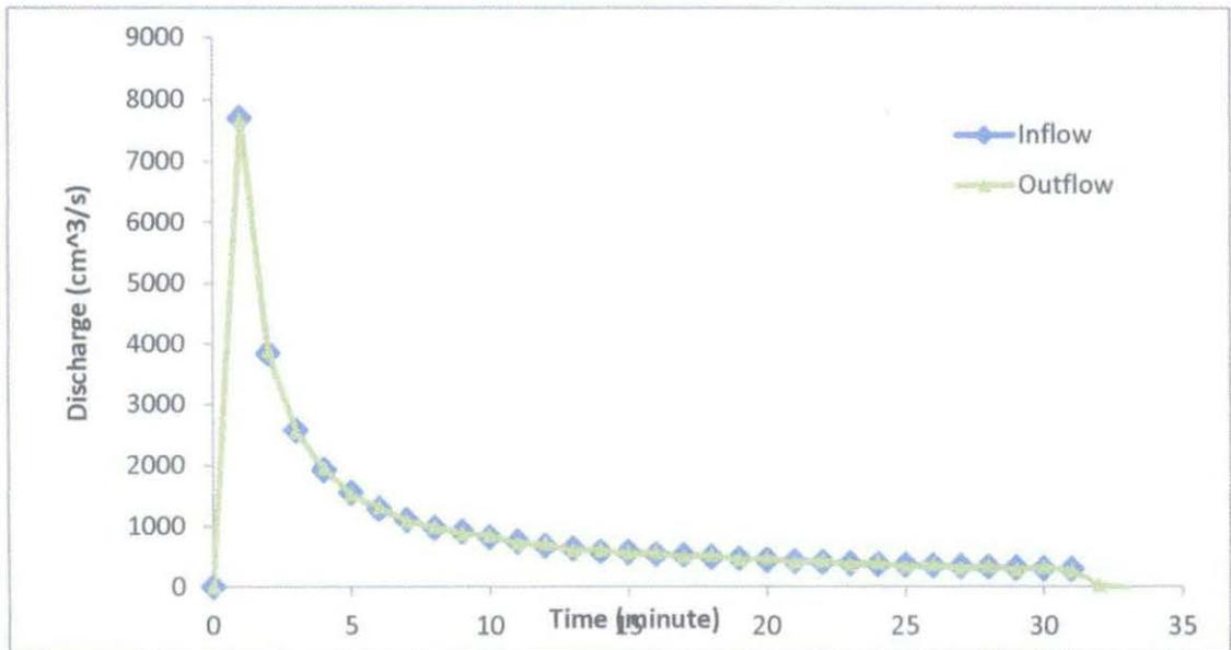
Figure 4.4: Discharge versus time for rotation one using Modified Puls Method
