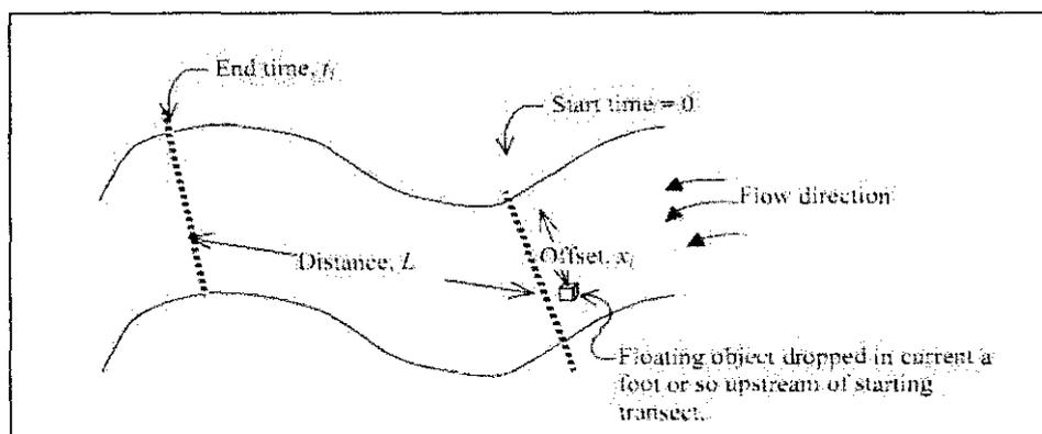
Figure 2.1: Float-method setup for measuring the stream/river surface velocity distribution. The velocity of section,  $i$ , is equal to  $L/t_i$ .
