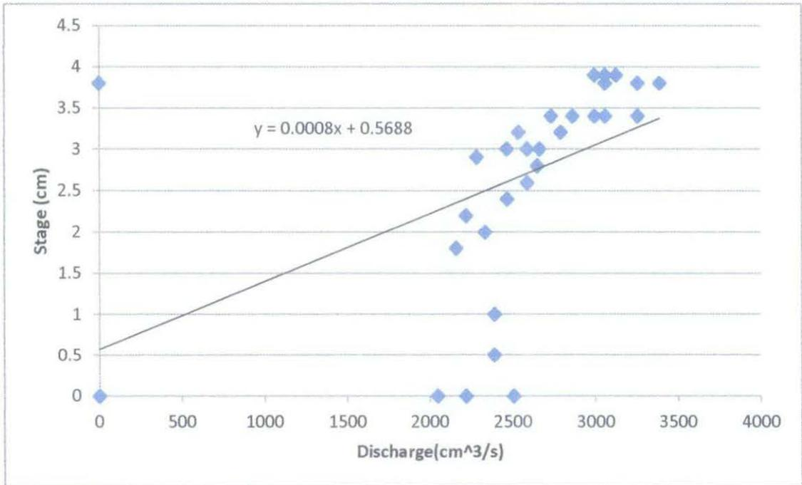
Figure 4.10: Stage versus discharge for rotation one
