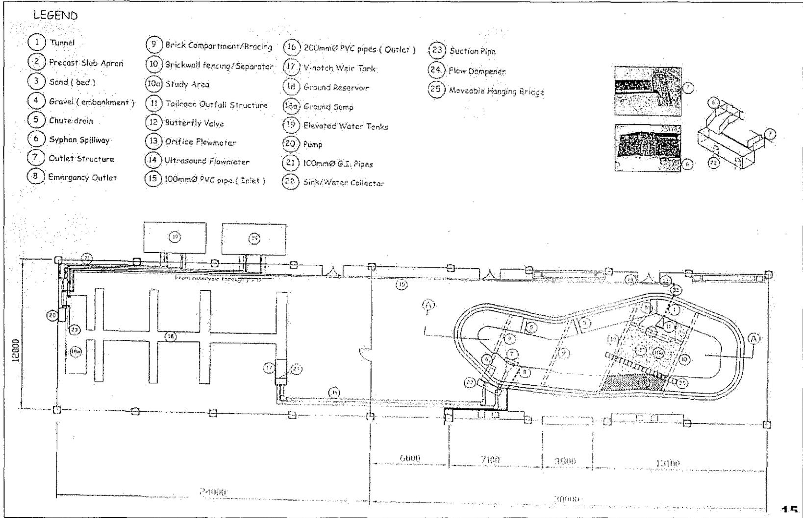
Figure 3. 2: Physical model of pond
