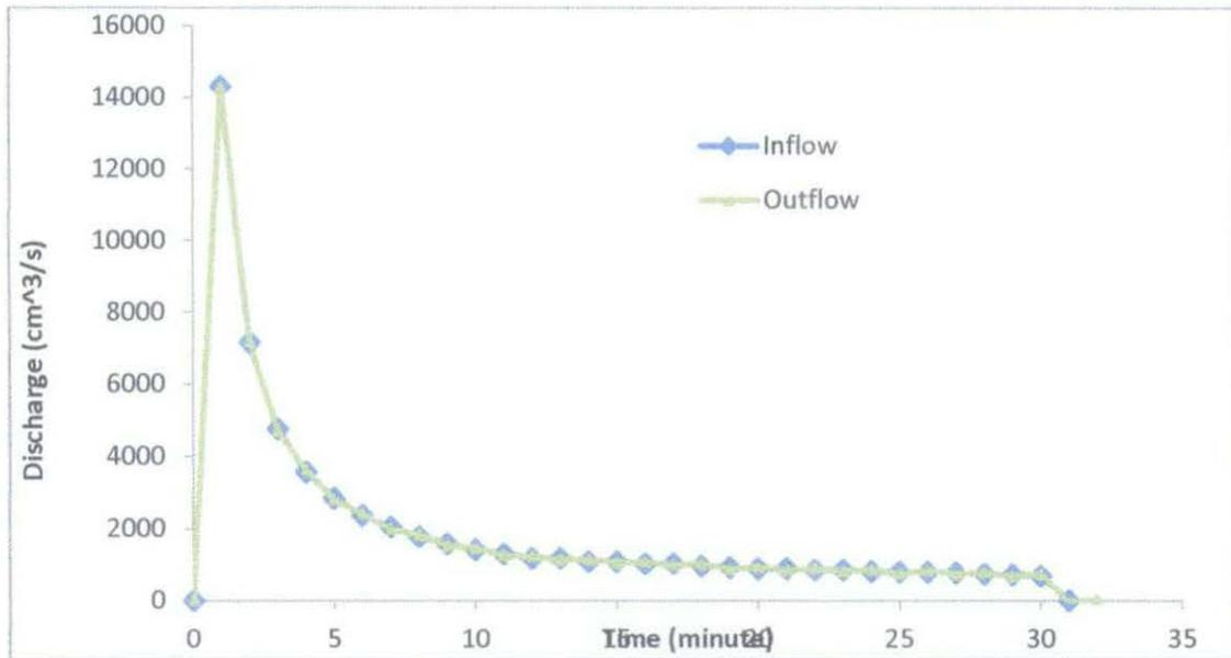
Figure 4.5: Discharge versus time for rotation two using Modified Puls Method
