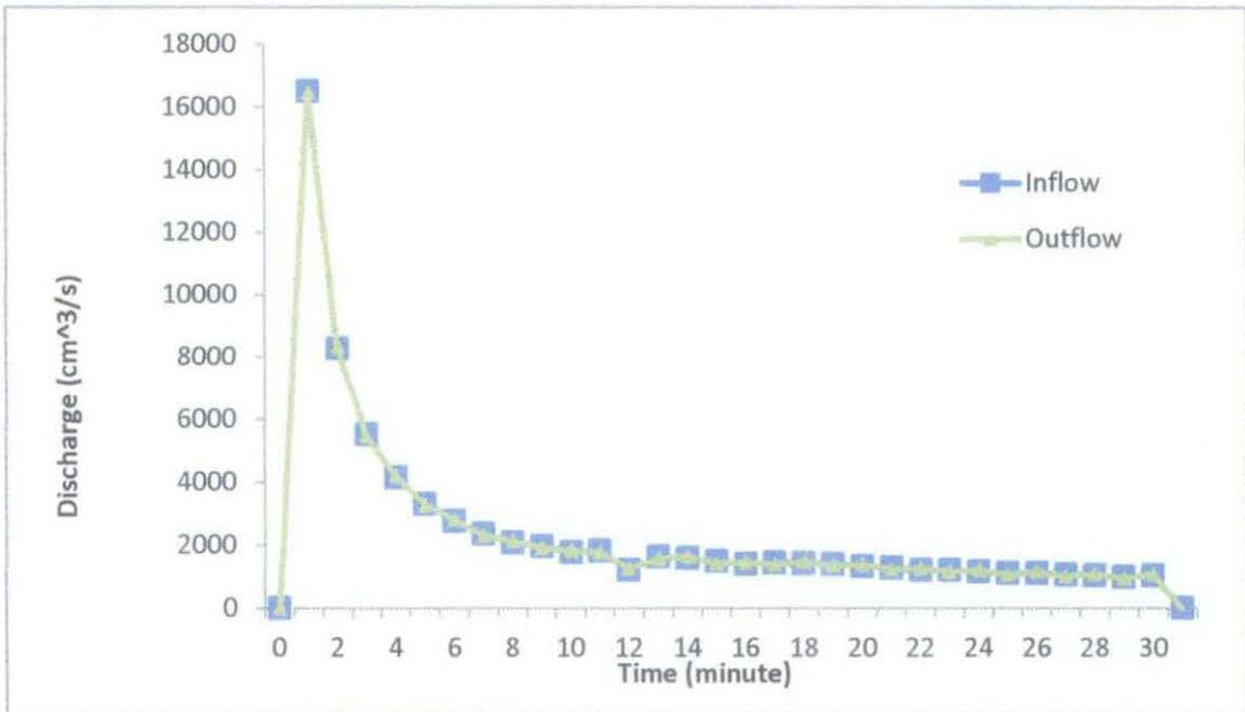
Figure 4.6: Discharge versus time for rotation three using Modified Puls Method
