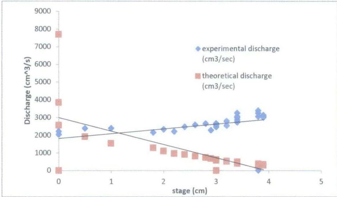
Figure 4.16: Comparison between calculated and experimental stage-discharge relationship
