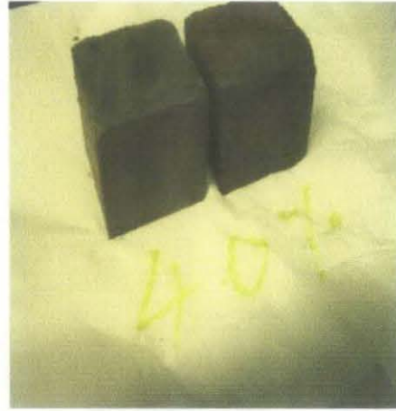
Figure 21: Cement cube with 40% ash
