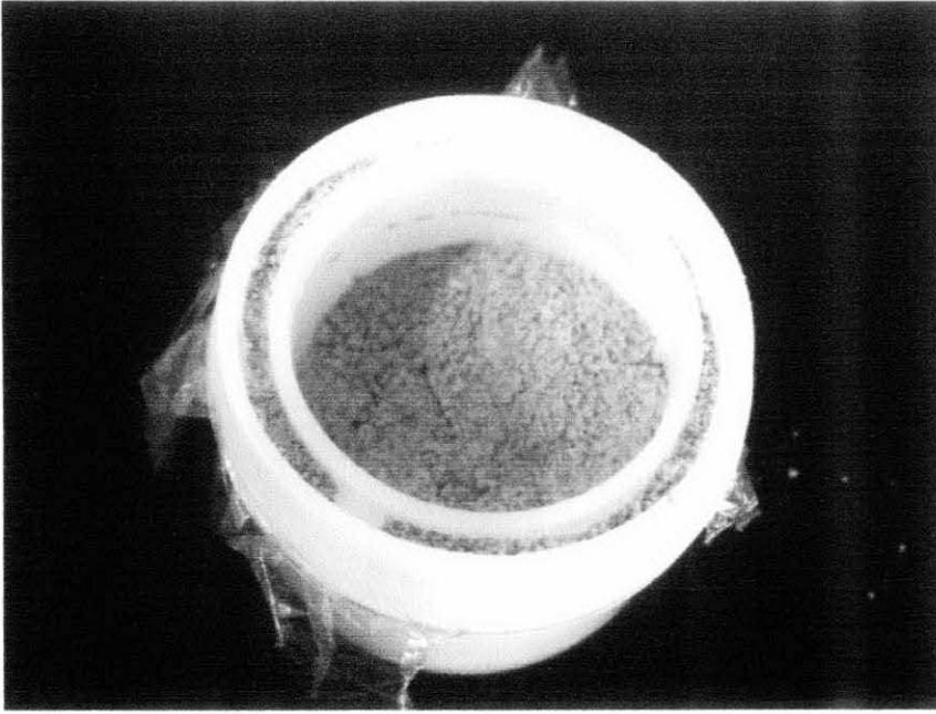
Figure 8: Lawin Tuff that has been grind into powder form
