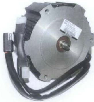
Figure 4.11: Example of brushless DC motor
