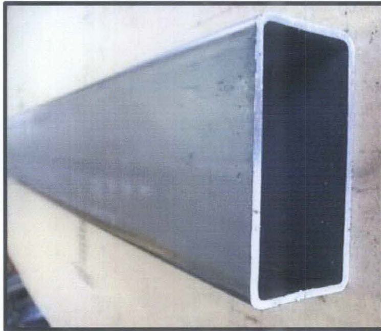
Figure 4.7: 1" X 2" rectangular mild steel tubing
