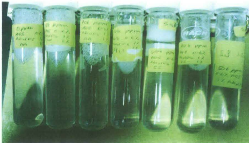
Figure 12: Brine condition (increasing salinity from left to right) with 1 wt % acrylic acid
