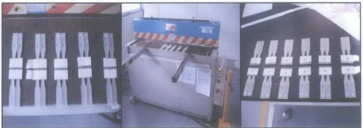
Figure 3.8: Sample preparation before FSW process.
