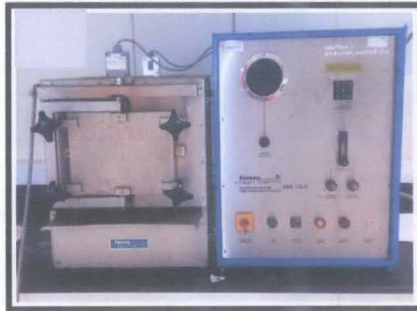
Figure 3.5: Tool heat treatment process in Tube Furnace.
