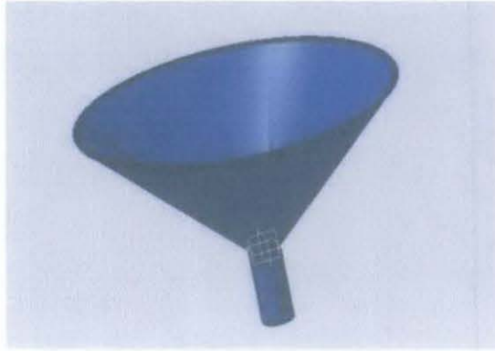
Figure 15 : Hopper Top (300mm Diameter cone with 20mm pipe outlet)
