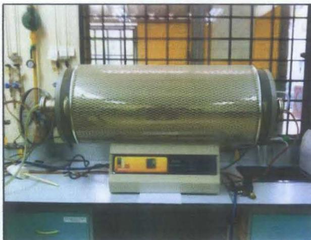
*Figure 7: Calcination process using furnace Carbolite*
