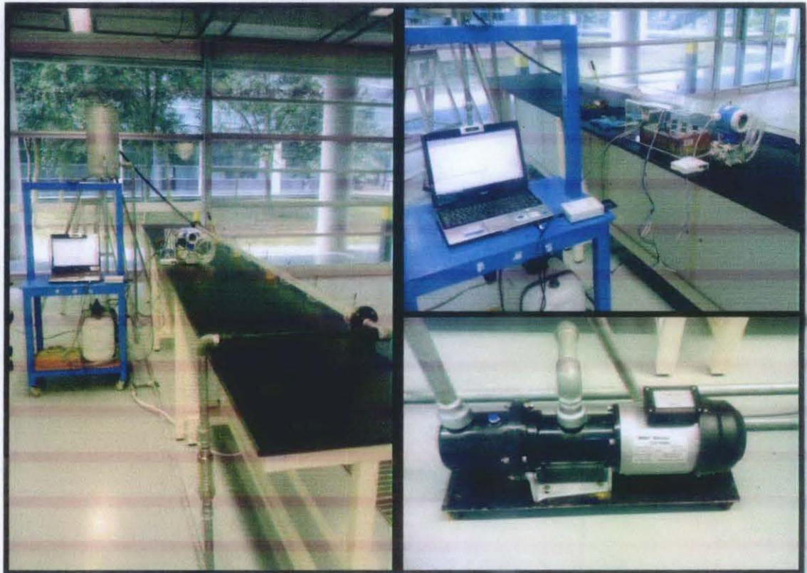
Figure 9: Complete setup of flow loop at block 18 laboratory.
