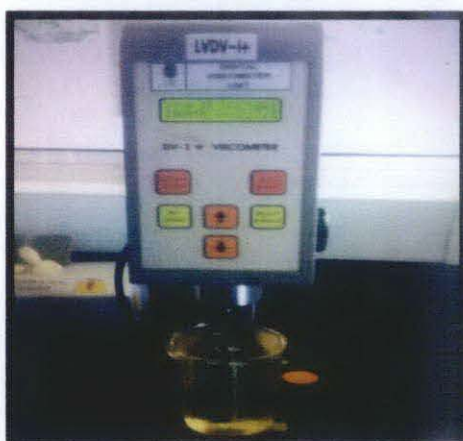
Figure 11: Digital viscometer used to measure Xanthan gum viscosity.
