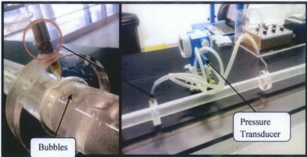
Figure 13: Test section and pressure transducer.
