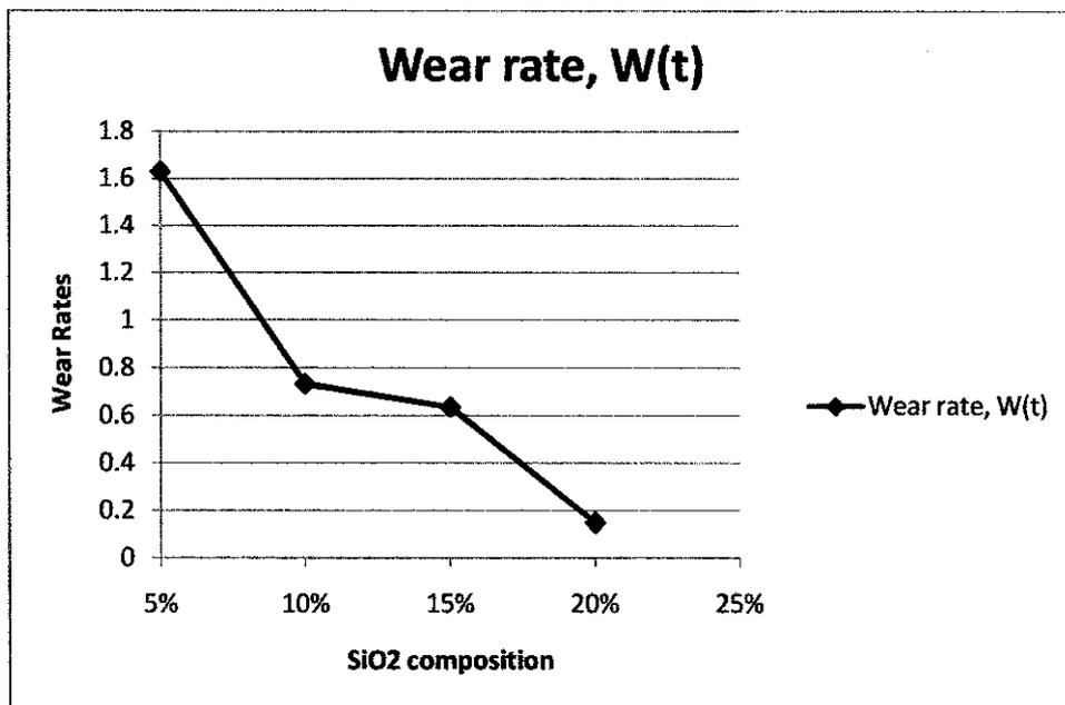
**Figure 22: Wear rate mm<sup>3</sup>/s 100 Newton Vs Nanosilica composition**
