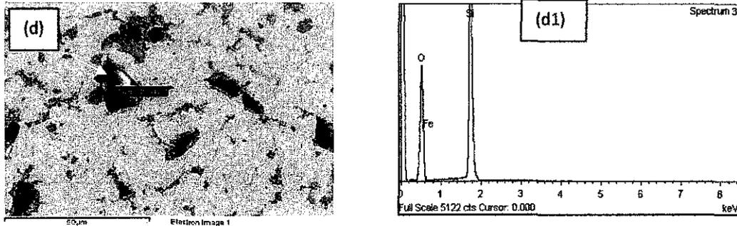
**Figures 16:** EDS (point) analysis of Fe-SiO<sub>2</sub> nanoparticles composites (*1100 °C sintering temperature*)
