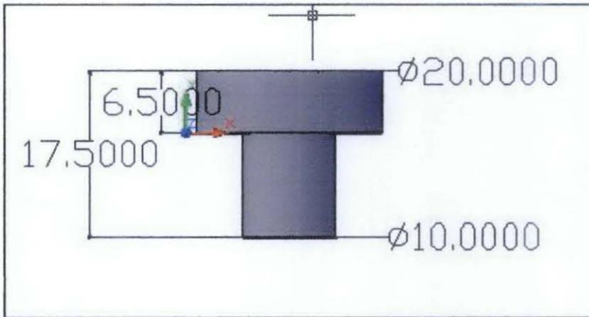
**Figure 19:** Side view with dimension holder for samples (pin)
