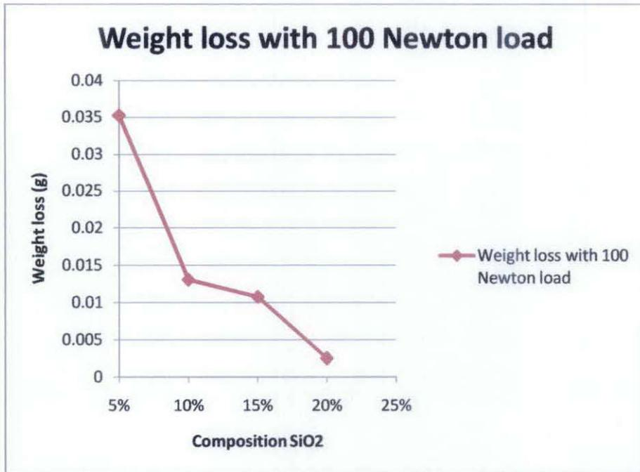
**Figure 20:** Weigh loss (g) 100 Newton Vs Nanosilica composition
