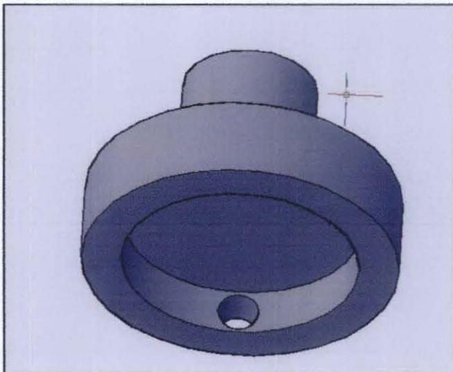
**Figure 10:** Holder for samples (pin)
