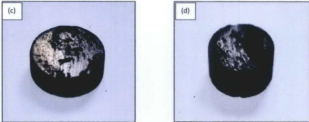
**Figure 21** : Sample of being wear of Fe-SiO<sub>2</sub> nanoparticles composites with (a) 5wt.% SiO<sub>2</sub>,(b)10wt.% SiO<sub>2</sub>, (c) 15wt.% SiO<sub>2</sub>, (d) 20wt.% SiO<sub>2</sub>. (100 Newton load )
