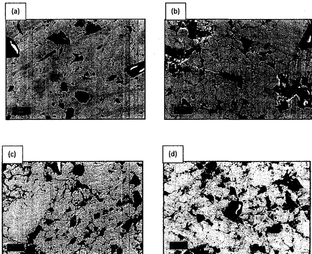
**Figure 14** : FESEM analysis of Fe-SiO<sub>2</sub> nanoparticles composites with (a) 5wt.% SiO<sub>2</sub>, (b) 10wt.% SiO<sub>2</sub>, (c) 15wt.% SiO<sub>2</sub>, (d) 20wt.% SiO<sub>2</sub>. (1000°C sintering temperature)
