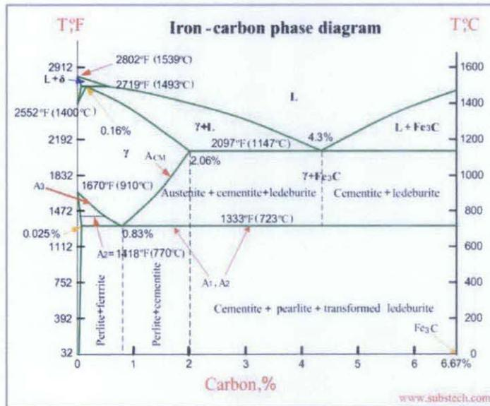
Figure 7 : The Iron - carbon phase diagram [15]
