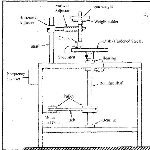
**Figure 12:** Schematic diagram of the pin-on-disk apparatus
