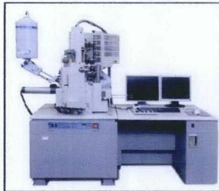
**Figure 8** : Field Emission Scanning Electron Microscopic (FESEM)
