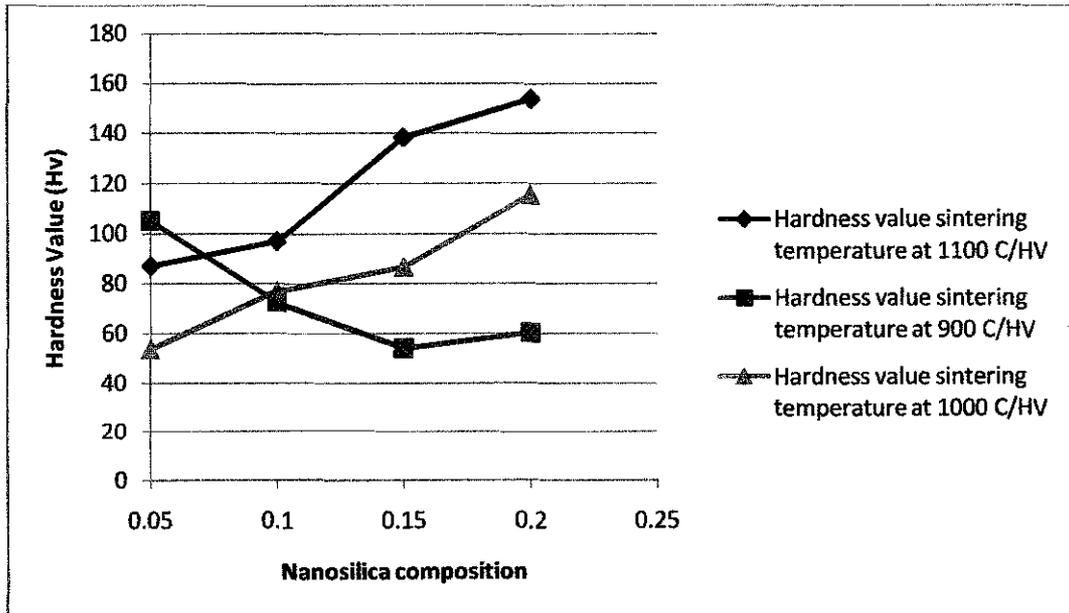
**Figure 17: Hardness (Hv) analysis Vs Nanosilica composition**
