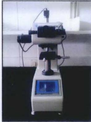
**Figure 9 :** Vickers Microhardness Tester
