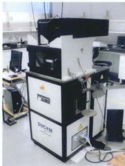
Figure 2.4: DUCOM Multi Specimen Tester
