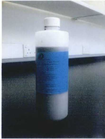
Figure 3.2: 1 micron DIAMAT Polycrystalline Diamond for polishing
