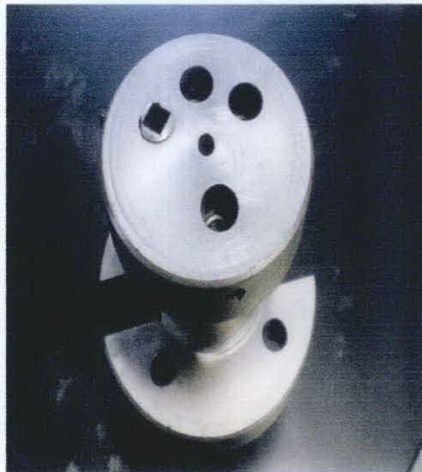
Figure 3.10: Sample holder for wear test.
