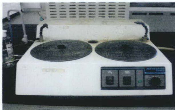
Figure 3.1: Grinding and polishing machine
