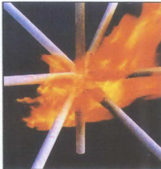
Figure 2.10: Pipes Covered With a Thin-Film Intumescent
