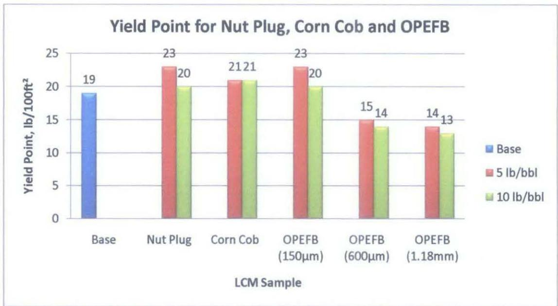
Figure 4.2 - Yield point for nut plug, corn cob and OPEFB in 5 lb/bbl and 10 lb/bbl
