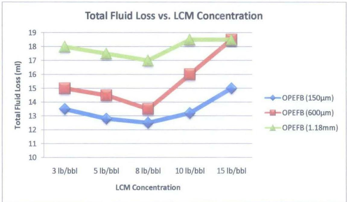
Figure 4.7 - Total Fluid Loss vs. LCM Concentration
