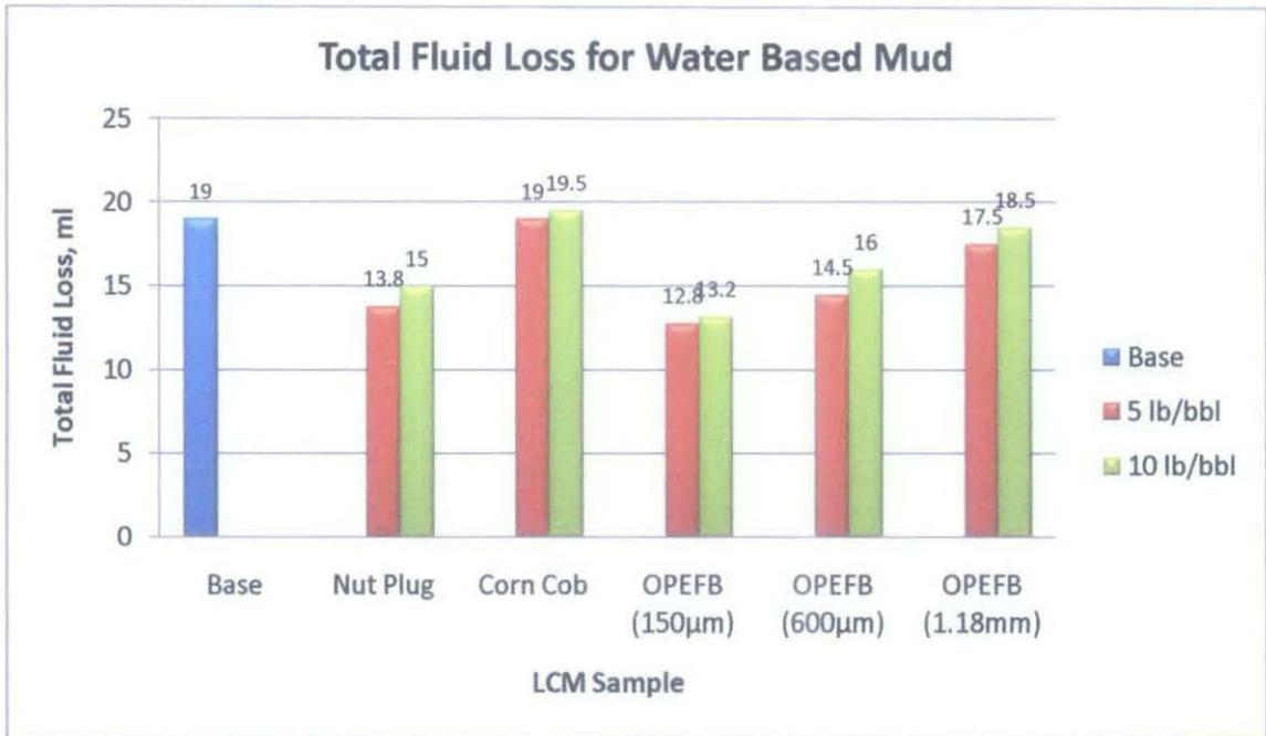
Figure 4.6 - Total fluid loss for water based mud
