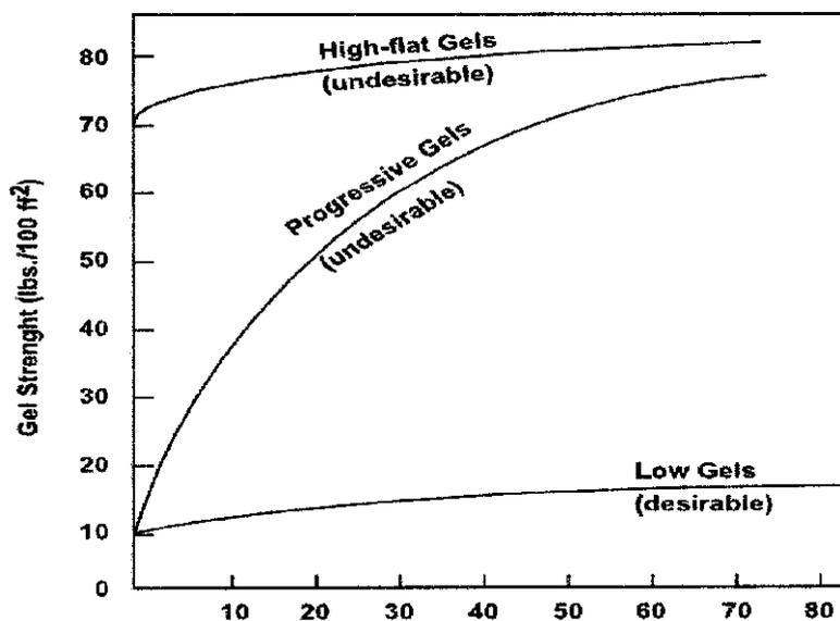
Figure 2.5 - Types of gel strengths diagram
