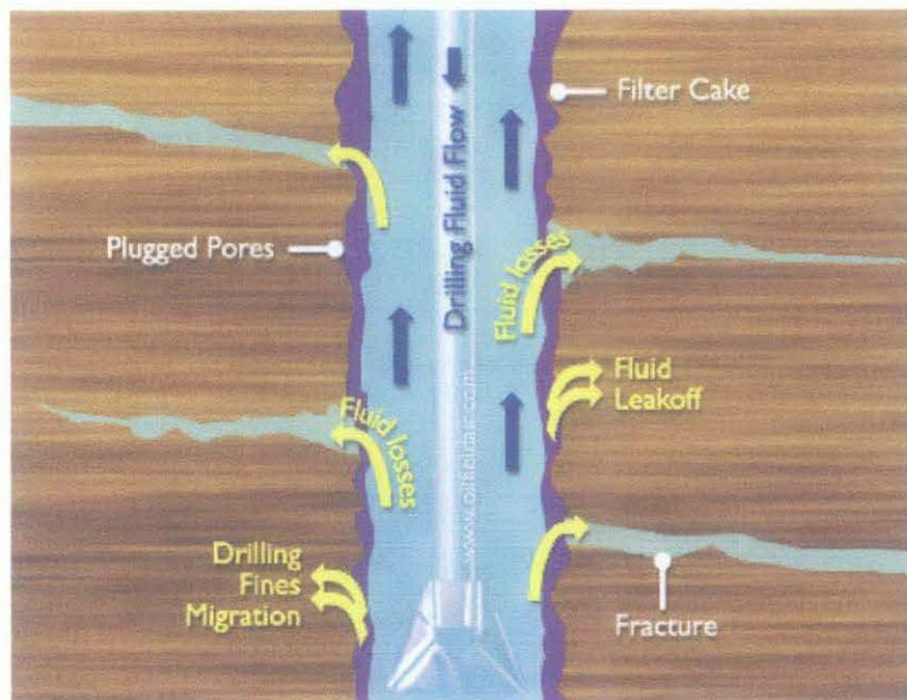
Figure 2.1 - Diagram illustrating the lost circulation
