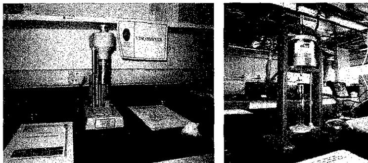
Figure 3.10 - FANN viscometer (left) and LPLT filter press (right)
