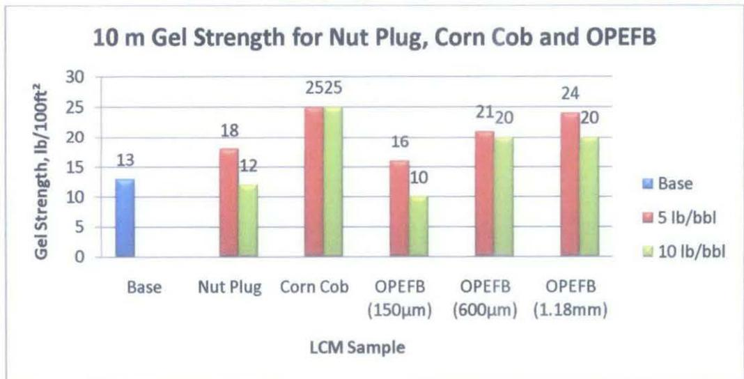
Figure 4.4 - 10-minute gel strength for nut plug, corn cob and OPEFB in 5 lb/bbl and 10 lb/bbl
