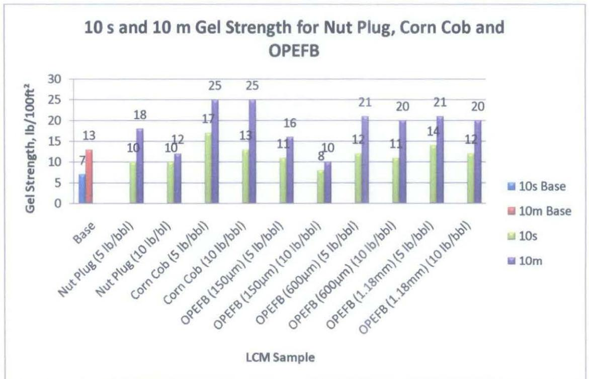
**Figure 4.5 - 10-second and 10-minute gel strength for nut plug, corn cob and OPEFB in 5 lb/bbl and 10 lb/bbl**
