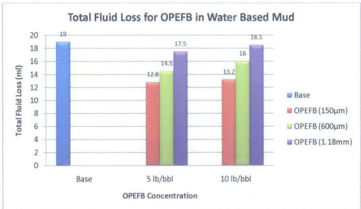
Figure 4.8 - Effect of LCM Concentration and Size Distribution on Total Fluid Loss for OPEFB in Water Based Mud
