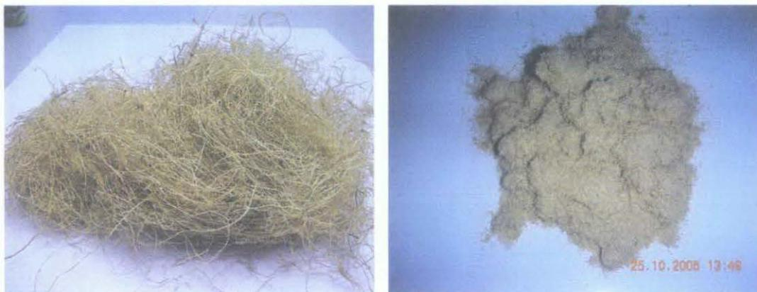
**Figure 2.10 - Oil palm empty fruit bunch (EFB) long fiber (left) and pulverized fiber (right)**
