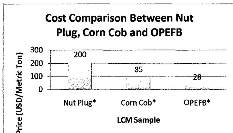
**Figure 2.12 - Cost comparison between nut plug, corn cob and OPEFB**
