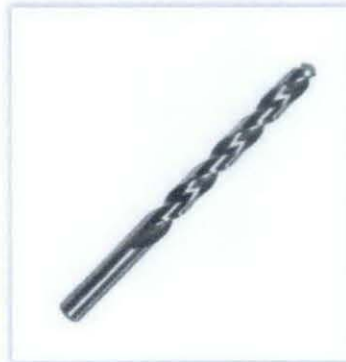
Figure 3.9: Drill Bit used during Process; HSS Twist Type Drill Bit.
