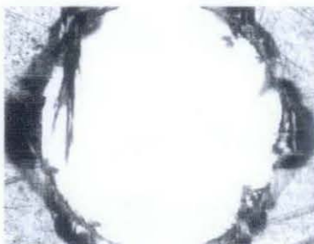
Figure 4.5: Splintering Observed around the Drill Area using Non Contact Machine.
