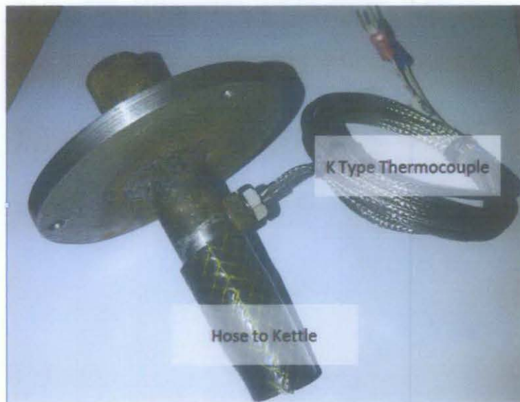
Figure 3.13 : Front view of the thermocouple bolted to the modified flange
