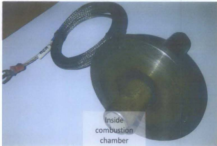
Figure 3.14 : Back view of the thermocouple bolted to the modified flange
