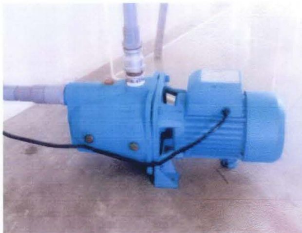
Figure 3.8: 1HP Water pump
