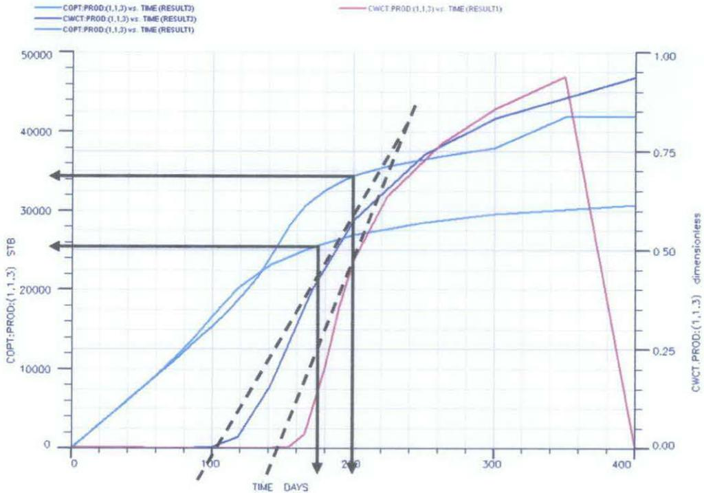
Figure 37: Oil Produced and Water Cut for layer 3 ( $M=0.5$  and  $2$ )
