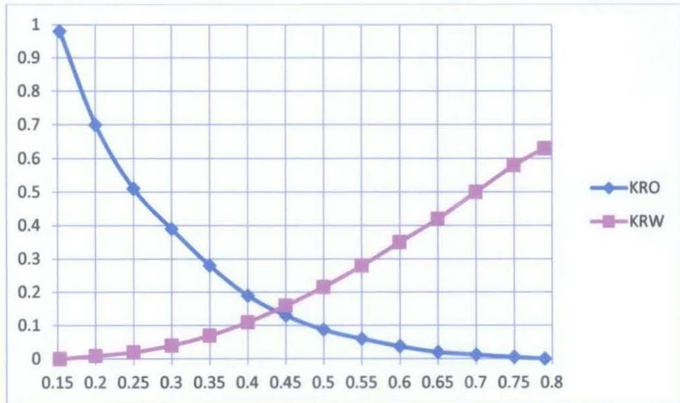
Figure 18: Relative Permeability versus Water Saturation
