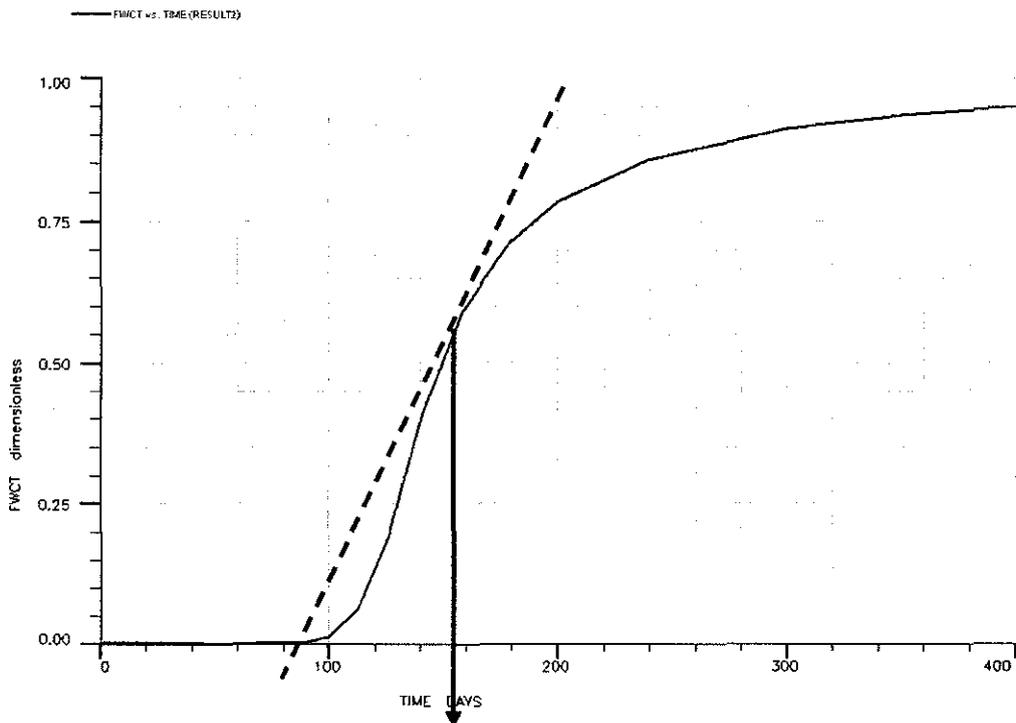
**Figure 25: FWCT versus Time (Base Case for Field)**
