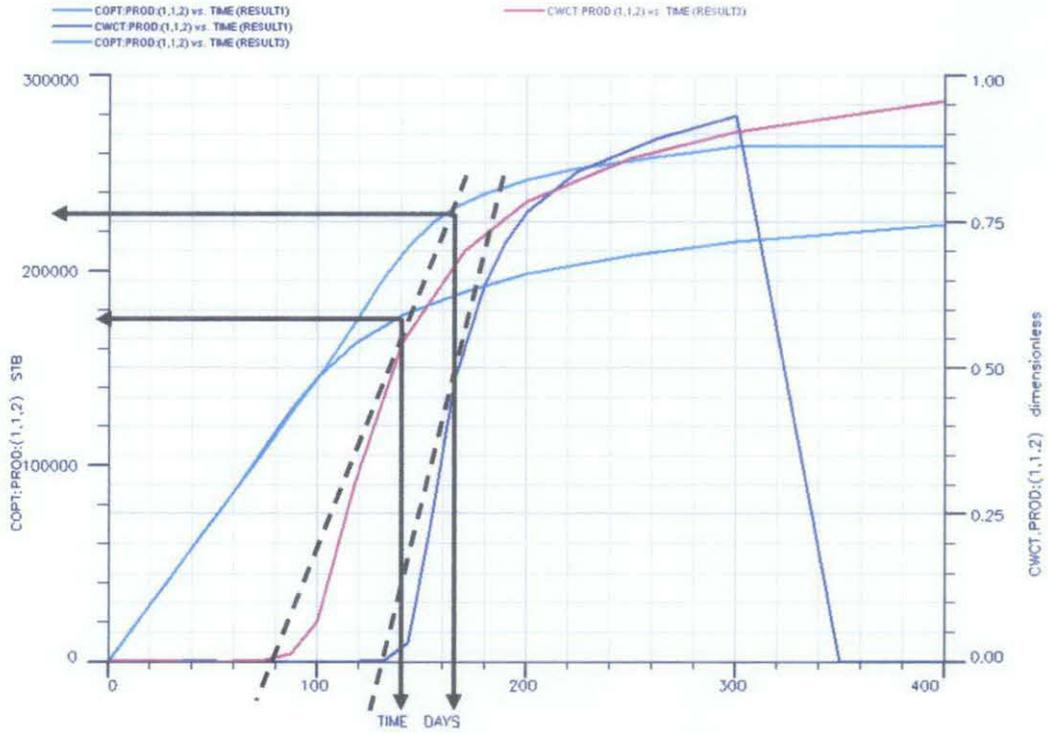
Figure 35: Oil Produced and Water Cut for layer 2 ( $M=0.5$  and 2)
