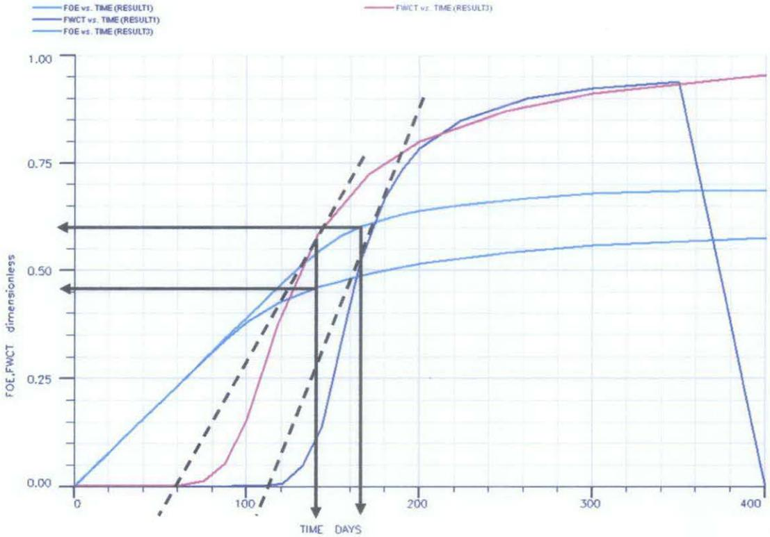
Figure 31: Oil Recovery Factor and Water Cut (M=0.5 and 2.0)
