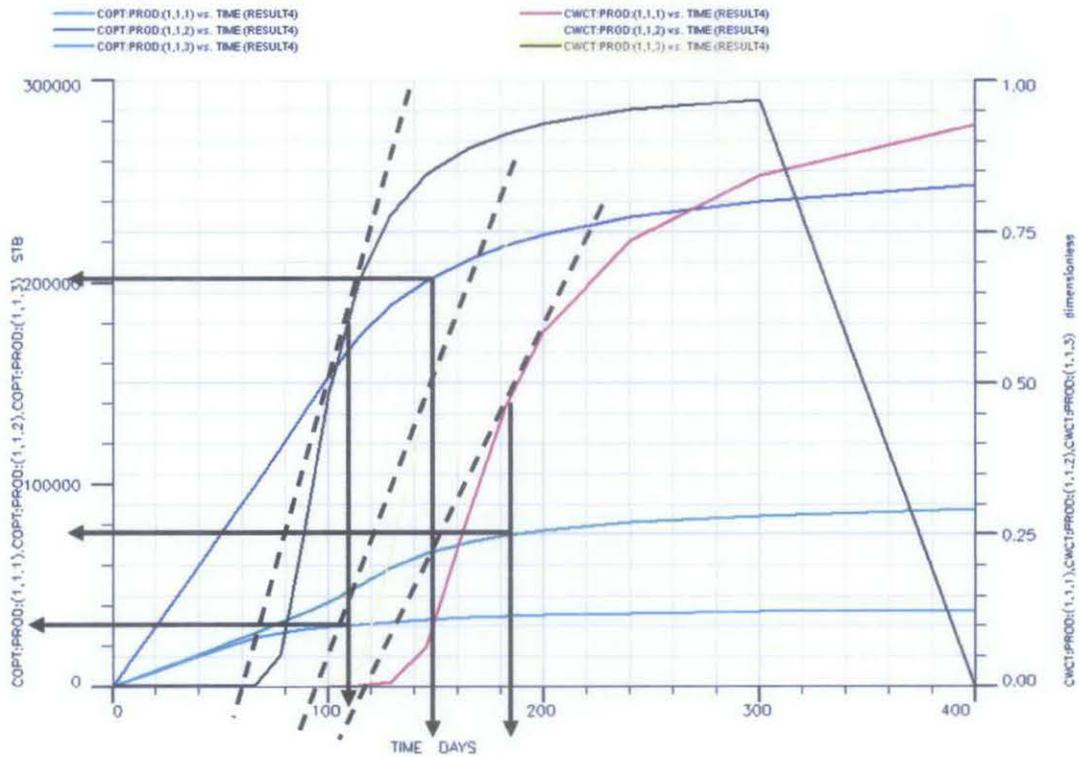
Figure 42: Oil Production and Water Cut for all layers (homogeneous model)
