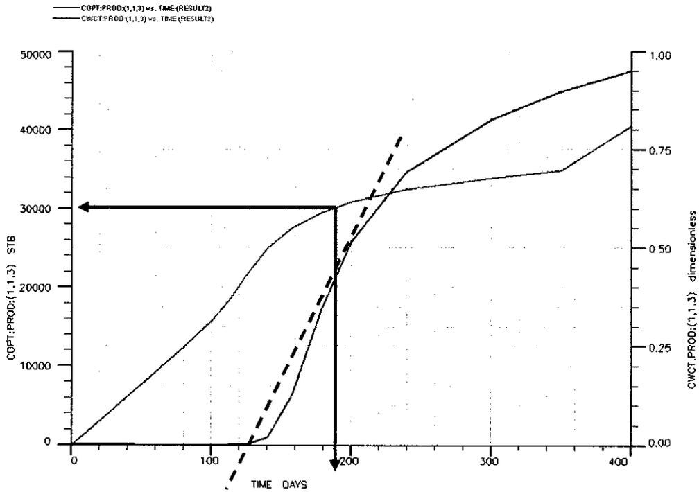
Figure 29: Oil Production and Water Cut for layer 3
