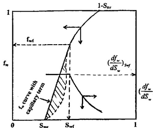
Figure 7: Fractional Flow Curves with Capillary Term
