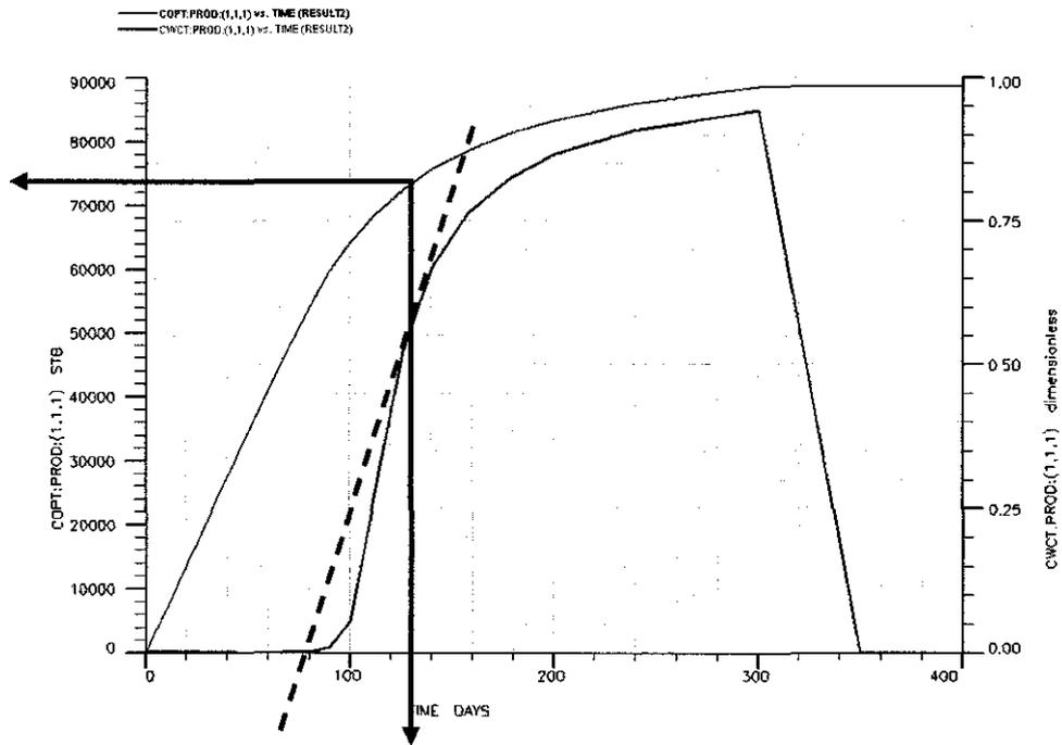
Figure 27: Oil Production and Water Cut for Layer 1
