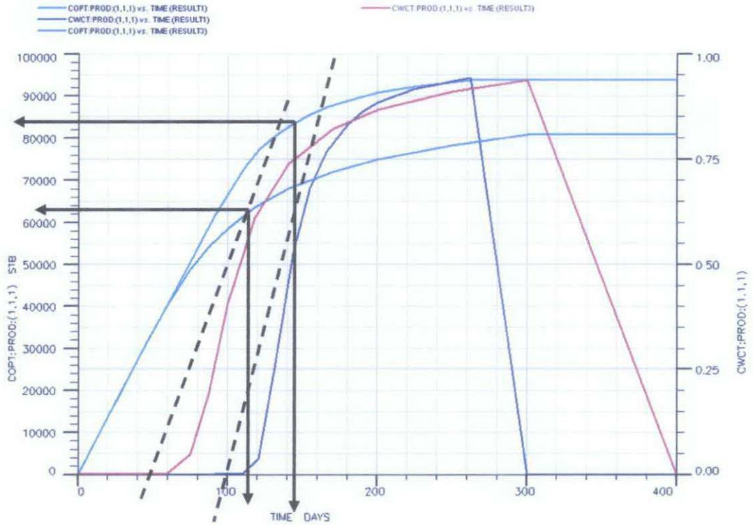
Figure 33: Oil Produced and Water Cut for layer 1 ( $M=0.5$  and 2)
