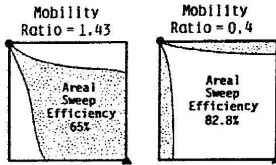
Figure 11: Areal Sweep Efficiency at Breakthrough
