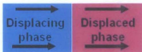
Figure 9: Illustration on Piston-like Displacement
