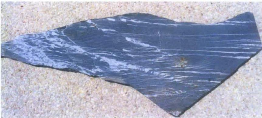
Figure 1.5 shows the Sungai Siput carbonate rock slab of thickness 20mm. The right hand side portion of this rock is taken to be used in this experiment because the rock lithology is more consistent compared to the left hand side of the sample where complex structure (white lines).
