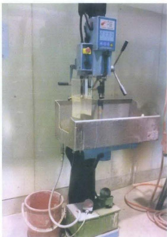
Figure 1.8 shows the Corex machine that will be used to make core plug of 1.5 in diameter
