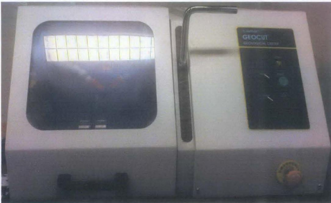
Figure 1.10above shows the Geo cutter that is being used to smoothen the surface of the core plug especially the edges of the core plug.
