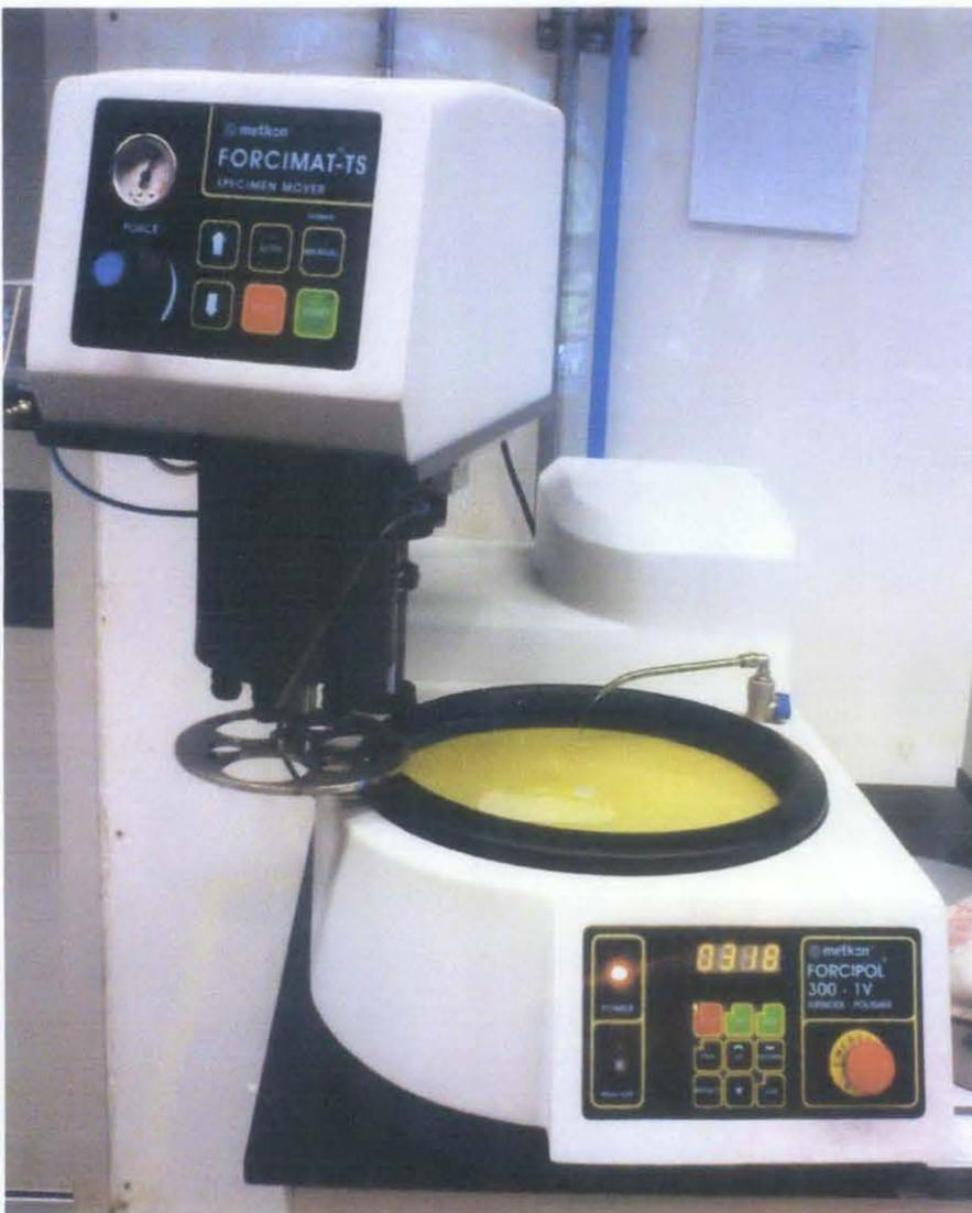
Figure 1.12 shows Forcipol and Forcimat that were used to smoothen the surface of the thin section. This process takes a long time as the surface need to be very smooth with thin layer which requires a slow process so that the rock sample will not crack.
