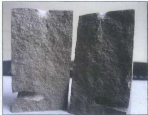
Side view of sample breakage- horizontal parent hole)
