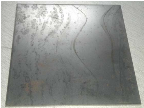
Figure 4(a) Before Sand Blasting
