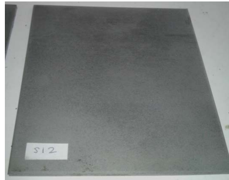
Figure 1(b) After Sand Blasting
