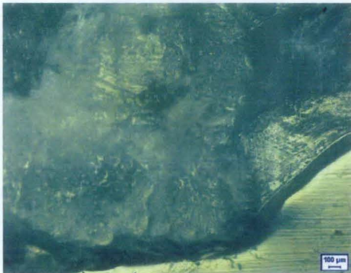
Figure 4.6 Region (b) which shows the structure of weld pool.
