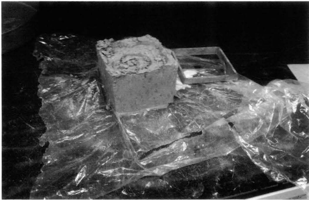
Figure 22 : Compacted soil is taken out to cut before putting in the shear box mould
