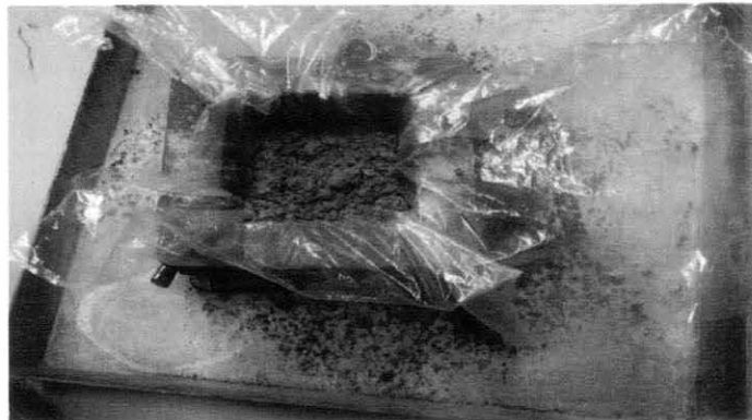
Figure 20 : Soil is placed 1/3 (1 layer) in compaction mould
