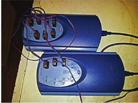
Figure 8: Data logger connected to thermocouples
