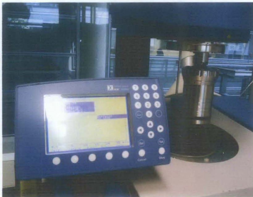
Figure 3: Bomb calorimeter experiment with jatropha oil
