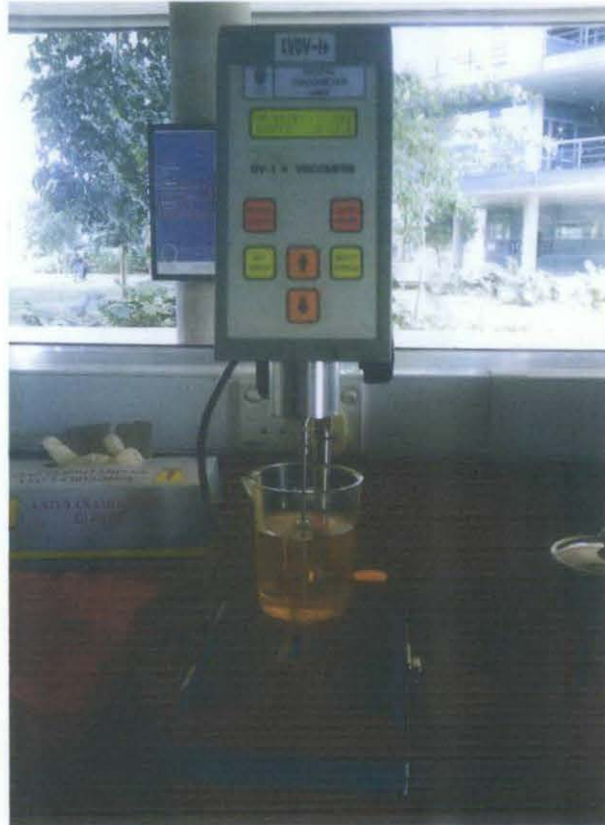
Figure 2: Kinematic viscosity experiment using jatropha oil
