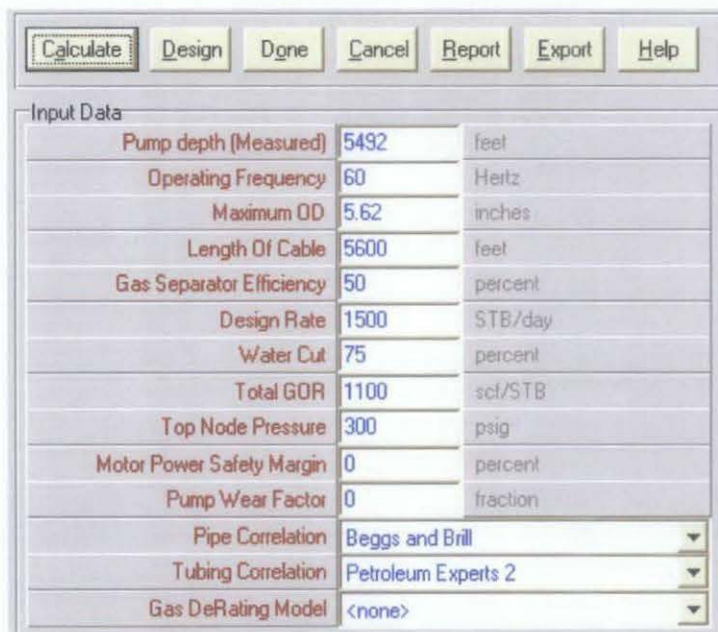
Figure 14 : ESP Design & Gas Separation Calculation
