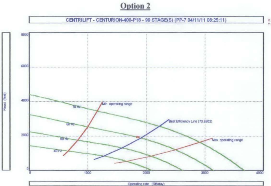
Figure 23 : Head Performance Curves of Centurion-400-P18 Pump at Different Frequencies
