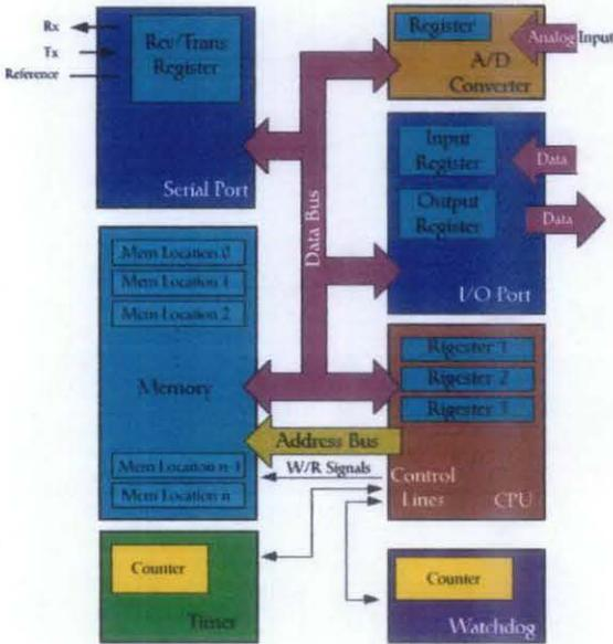
Figure 1: Microcontroller basic block diagram
