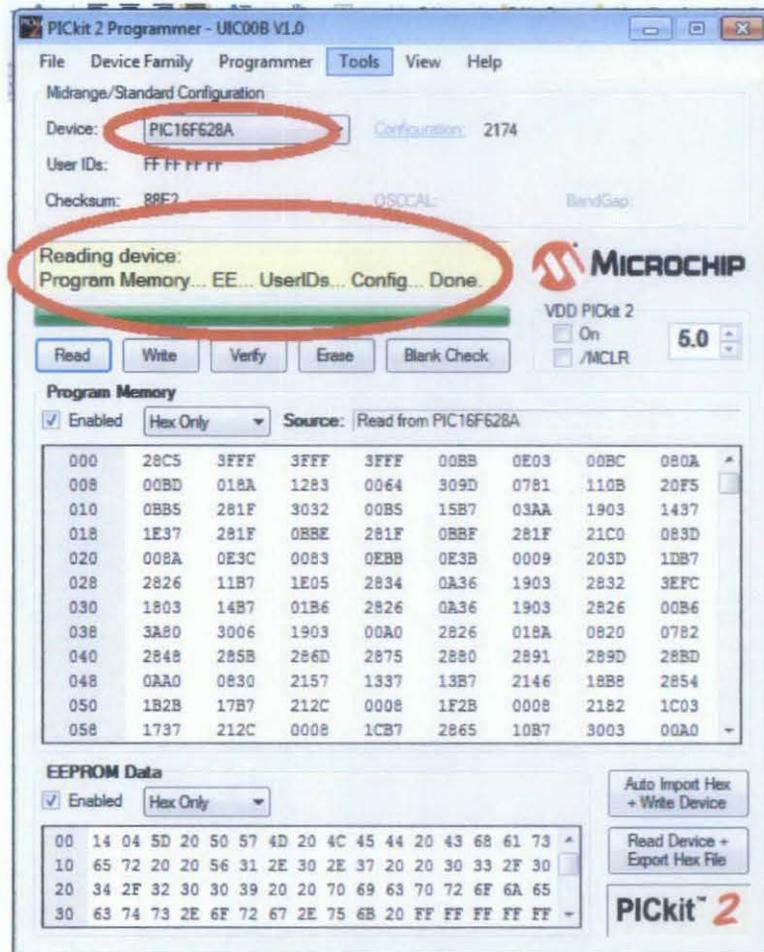
Figure 14: PICKit 2 Programmer interface after connection with main board are made
