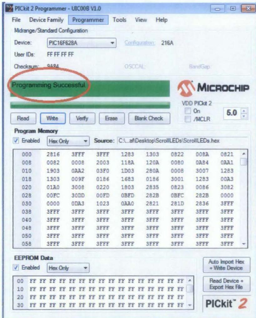
Figure 15: Load HEX file into PIC16F628A
