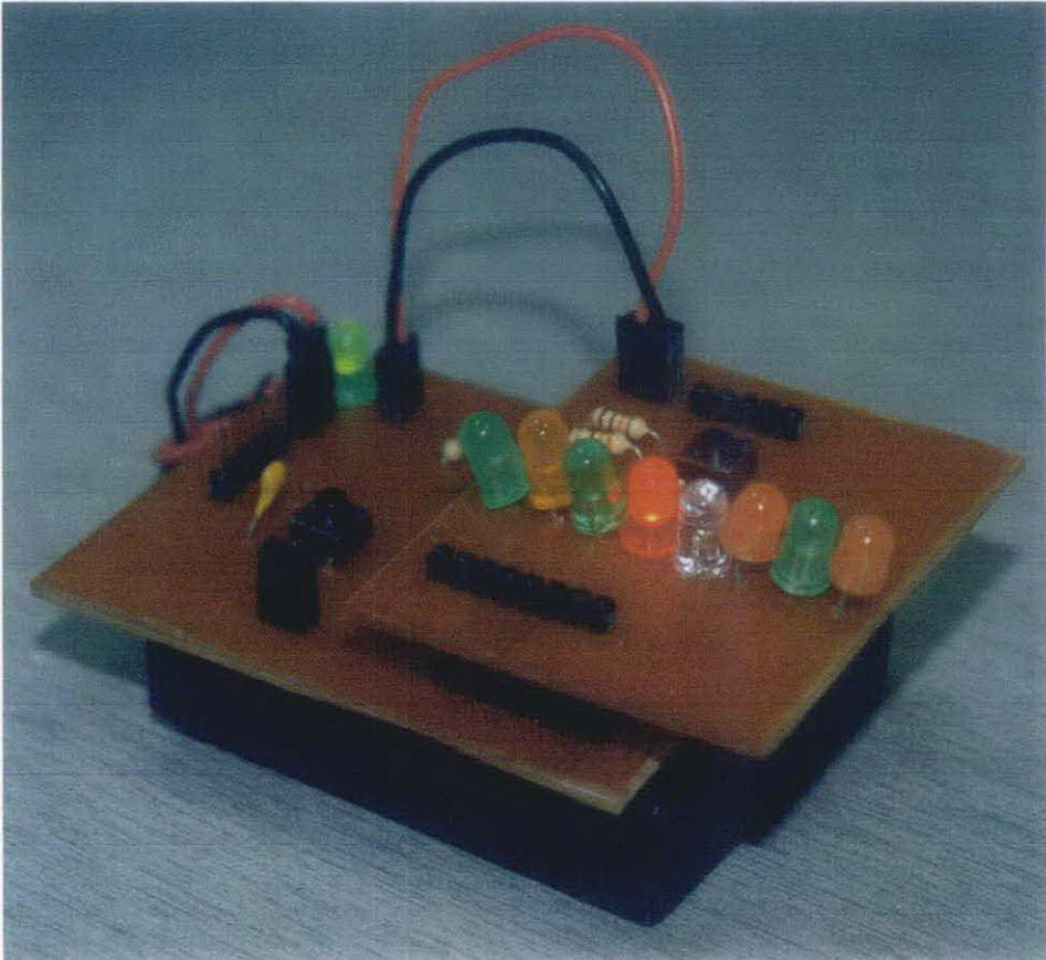
Figure 18: Add-on board mount on main board
