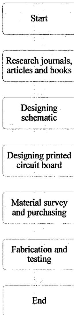
Figure 3: Process of designing and fabricating a PIC16F628A small prototyping board
