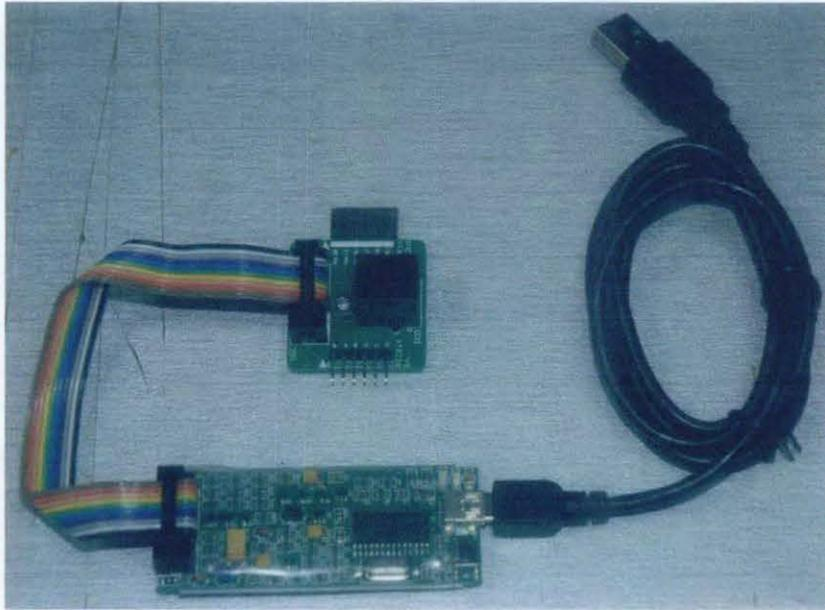
Figure 12: PIC USB Programmer
