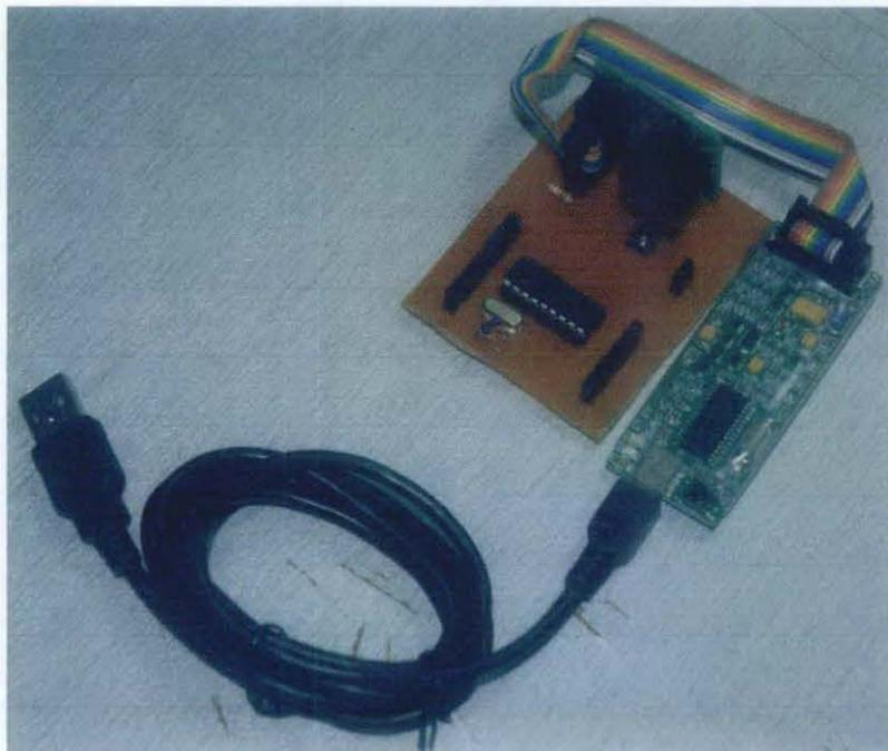
Figure 13: Connected main board with programmer
