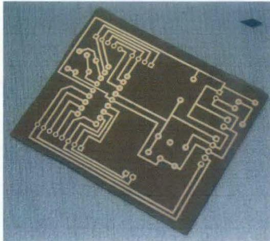
Figure 9: Conductive pathways on the PCB
