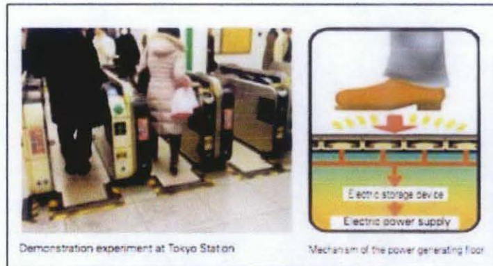
Figure 2 : Energy Generating Floor System [6]
