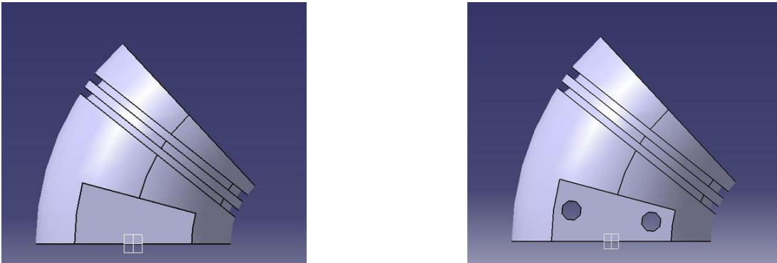
Figure 23: Before and after drilling of piston pin hole.
