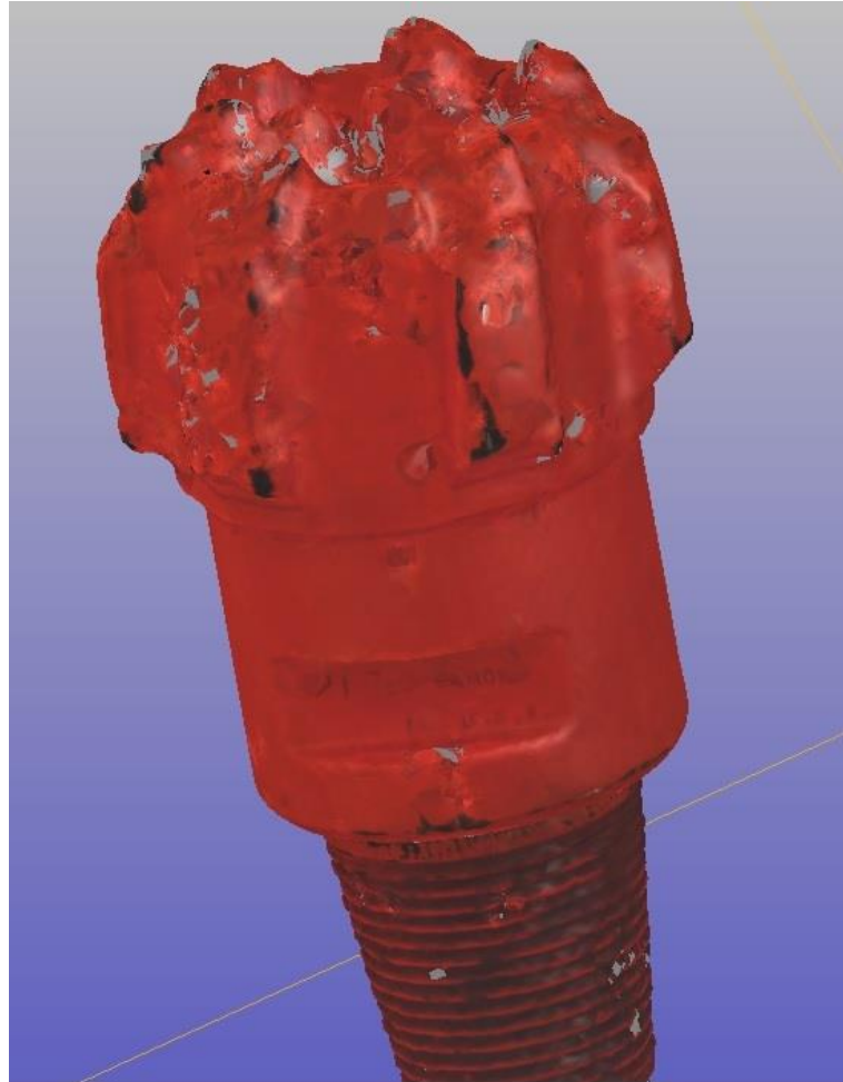
Figure 18: Cloud model of PDC Drill Bit.
