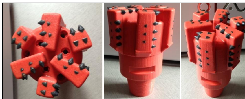
Figure 36: Prototype of improve design PDC bit.
