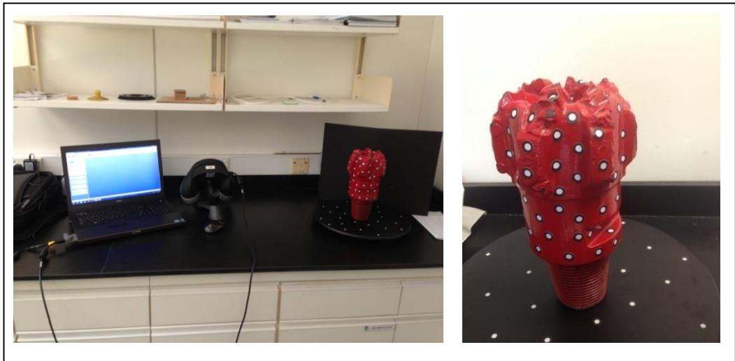
Figure 10: 3D scan setup.
