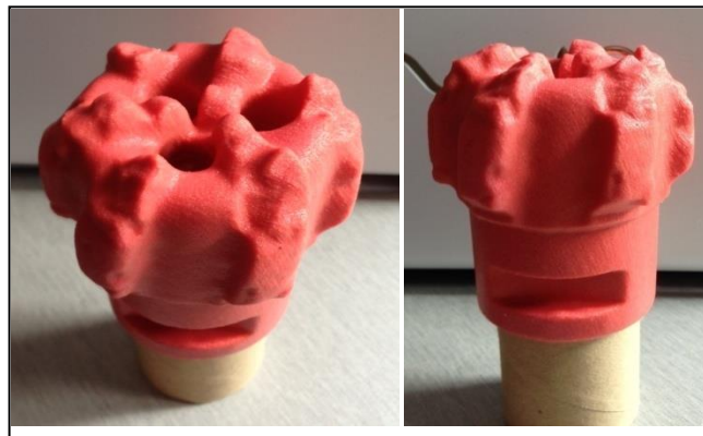
Figure 34: Prototype of RE worn PDC bit.
