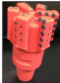
Figure 35: Prototype of like new design PDC bit.
