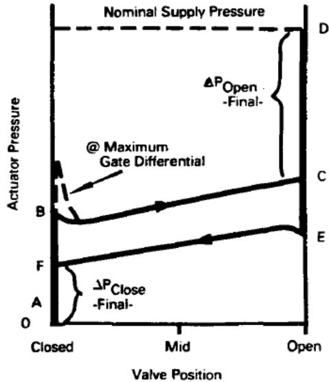
Figure 35. Gate valve behavior from Cadlao field [19]
