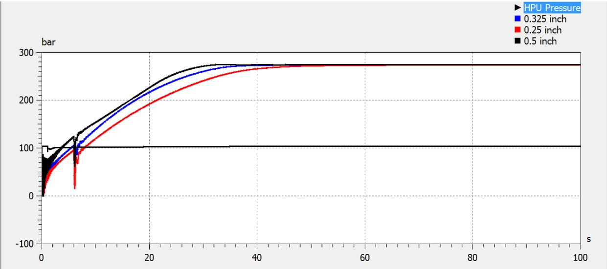
Figure 37. Umbilical line hose diameter (inch) vs. steady state time (s)
