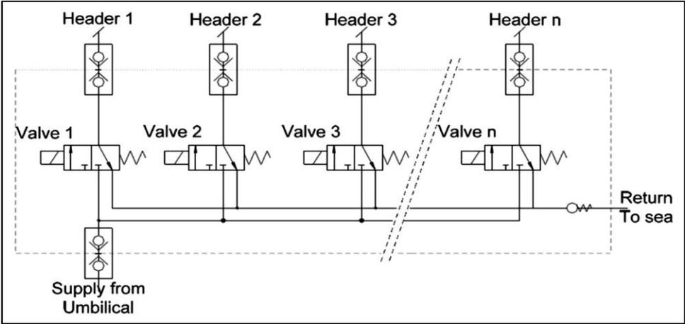
Figure 18. Schematic diagram of Subsea Control Module [7]
