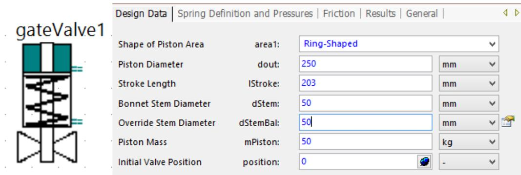
Figure 24. Gate valve model and parameters
