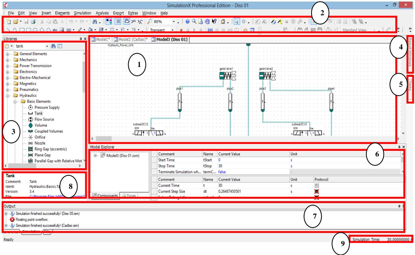
Figure 13. SimulationX GUI overview
