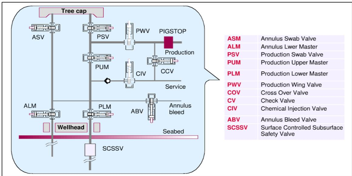
Figure 5. Subsea Production Valves [9]
