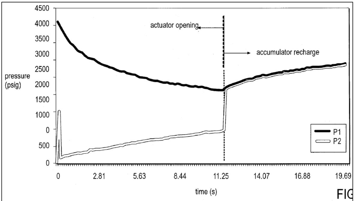
Figure 10. Typical valve signatures for a non-leaking system during actuator opening and recharge [15]
