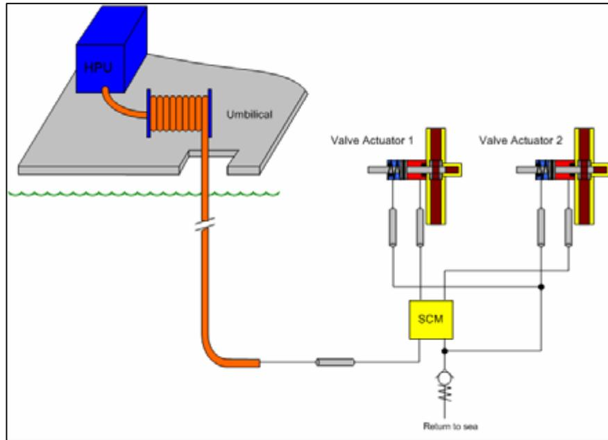
Figure 15. Hydraulic control system sketch [7]
