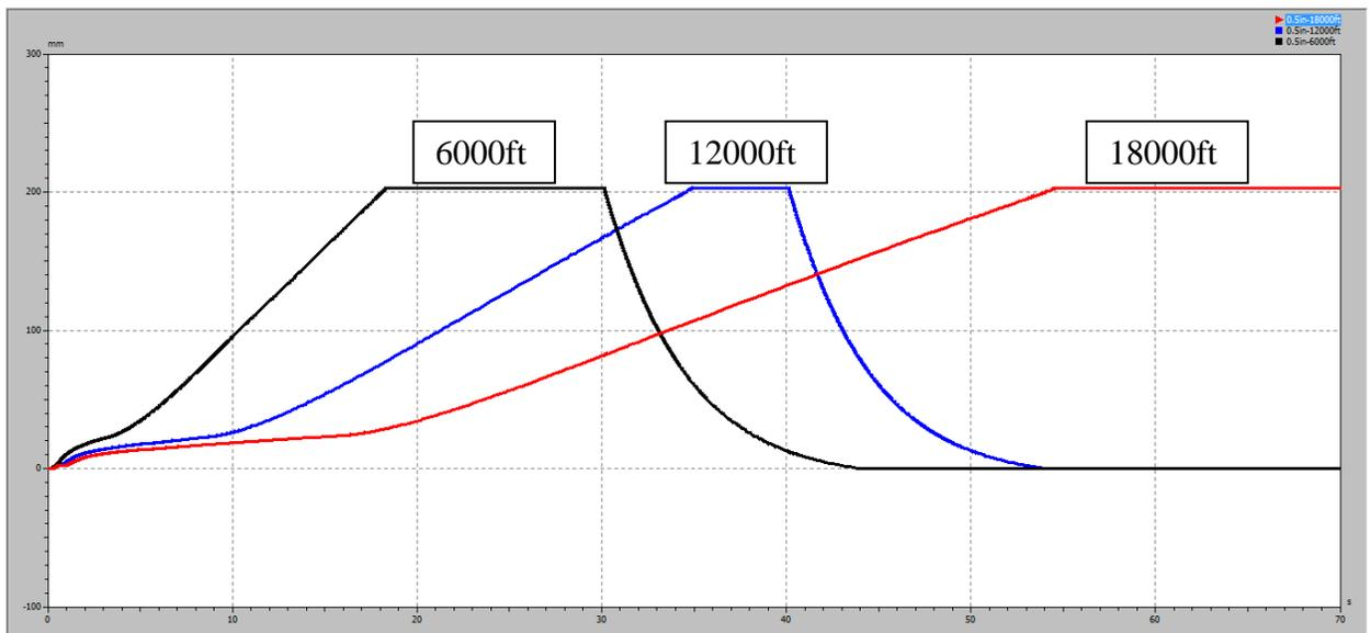
Figure 40. Effect of hose line length, valve actuator stroke (mm) vs. time (s)
