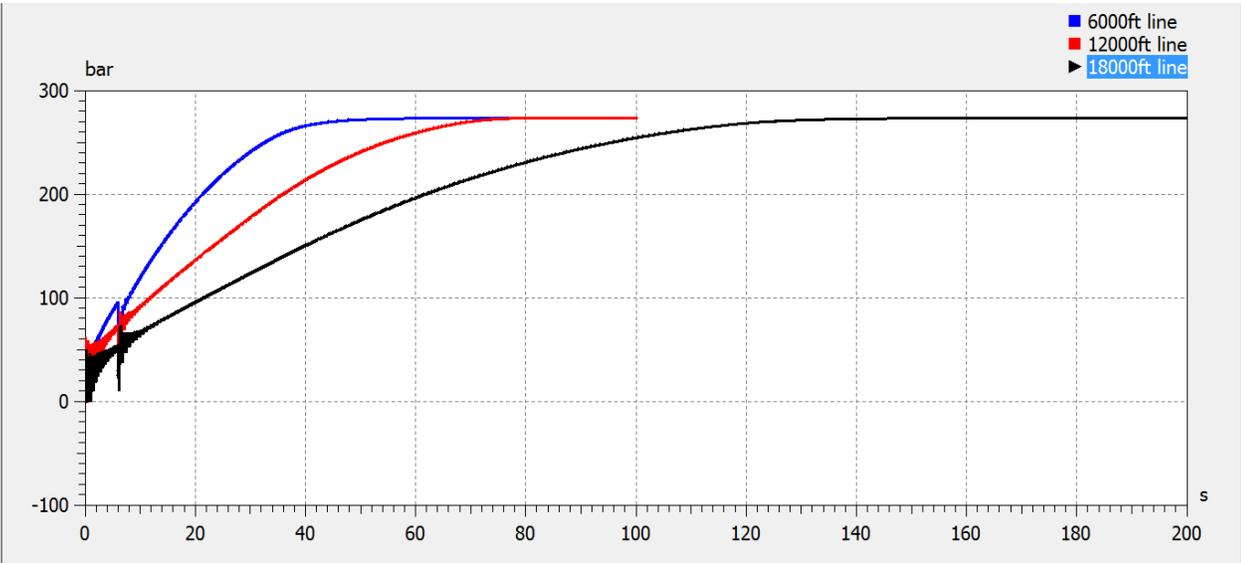
Figure 38. Effect of varying hose line length to the signal time
