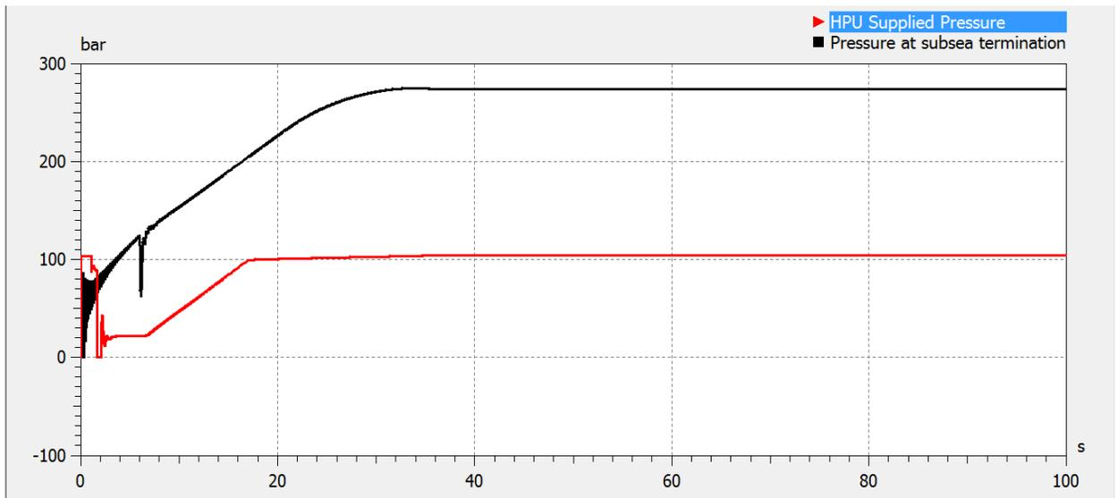
Figure 36. Umbilical hose line pressurization
