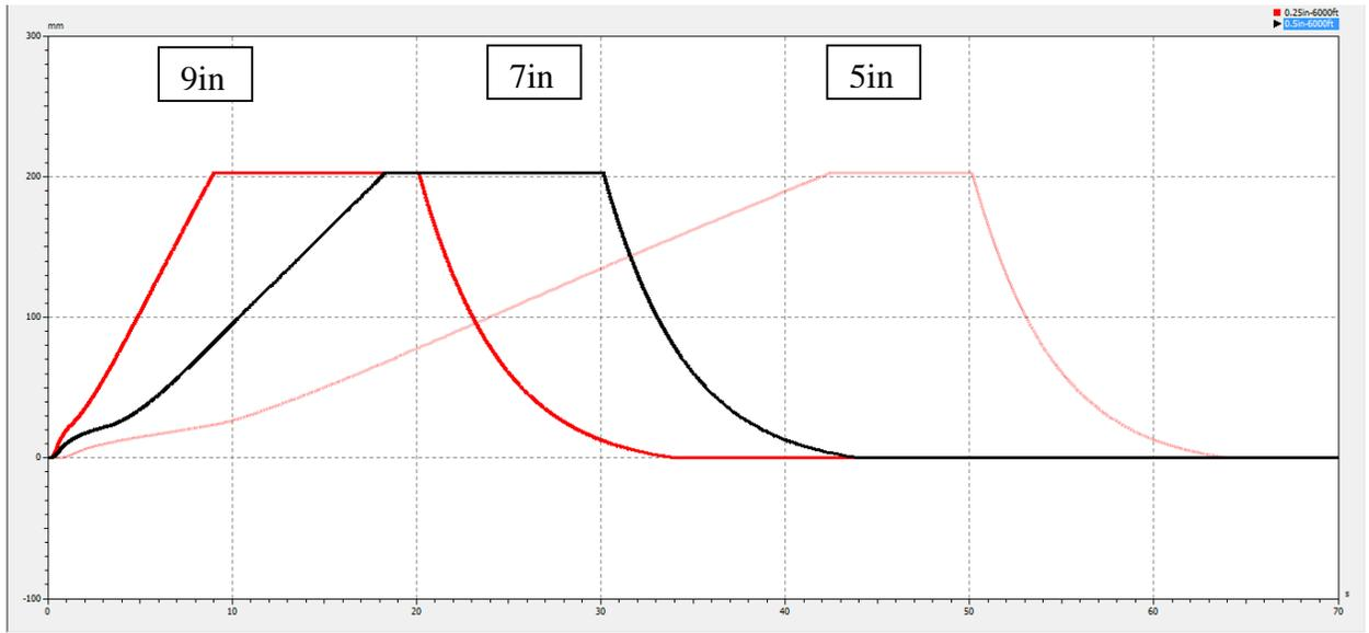
Figure 41. Effect of hose line diameter, valve actuator stroke (mm) vs. time (s)
