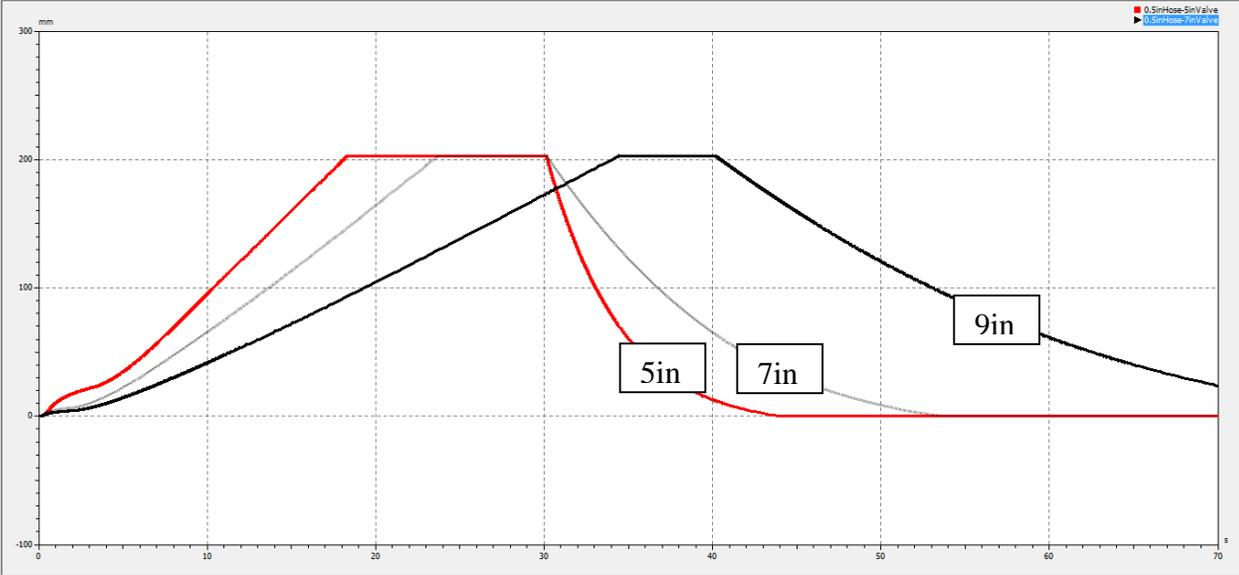
Figure 42. Effect of valve size on signal response, valve actuator stroke (mm) vs. time (s)
