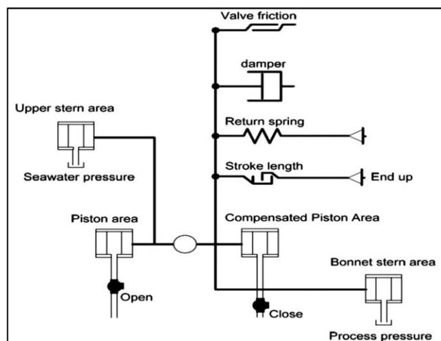
Figure 23. Gate Valve model [7]
