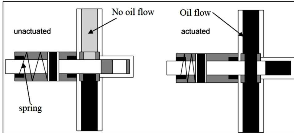
Figure 22. Gate Valve in Close and Open positions [7]
