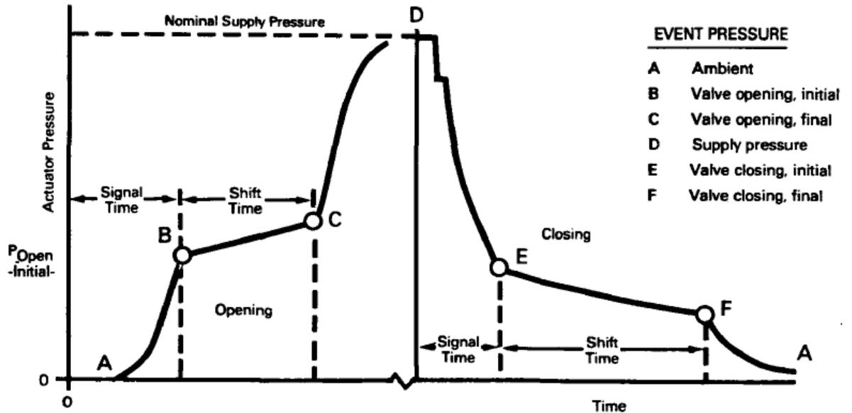
Figure 29. Signal & Shift response time [19]
