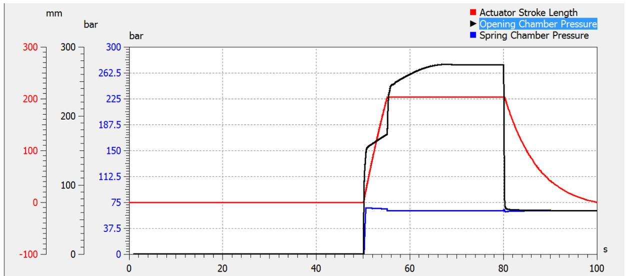
Figure 33. Pressure response curves when opening a 4 inch gate valve #1
