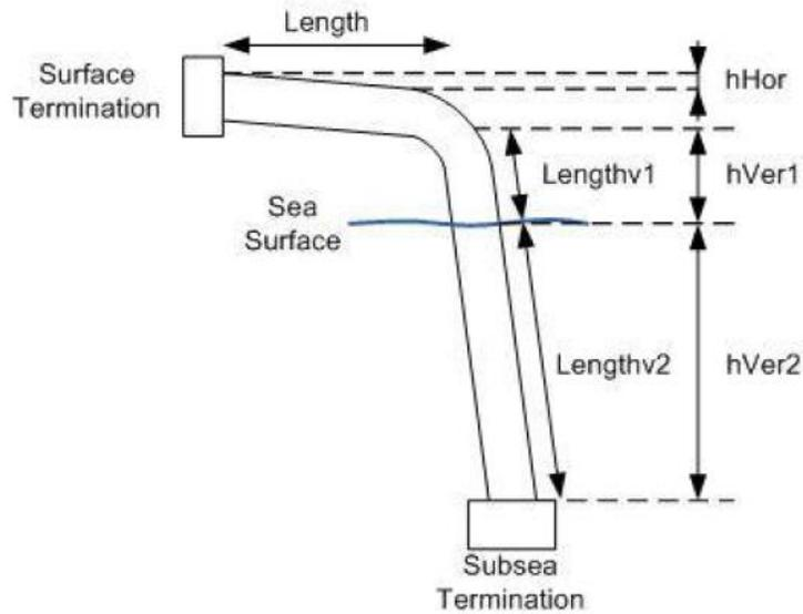
Figure 26. Umbilical line geometry configuration [17]
