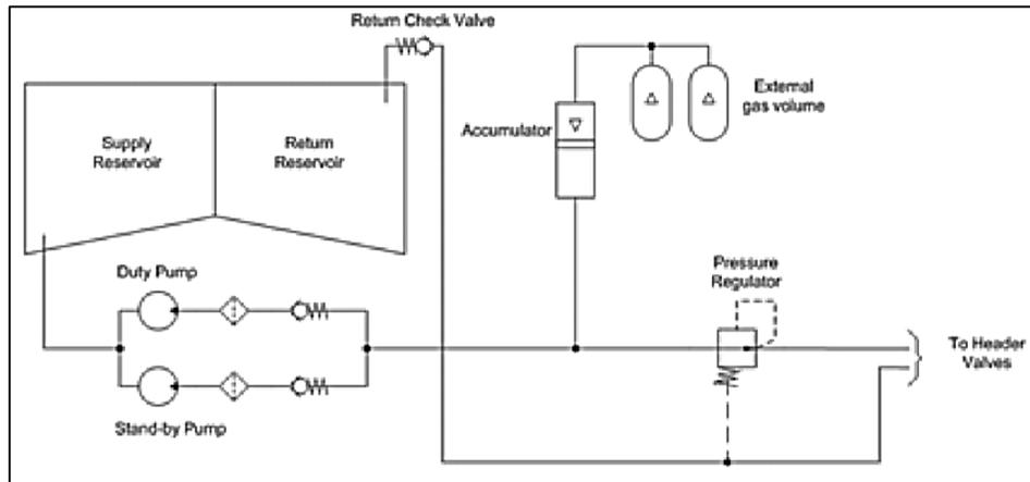
Figure 16. Simplified schematic diagram of a pumping unit (HPU) [7]
