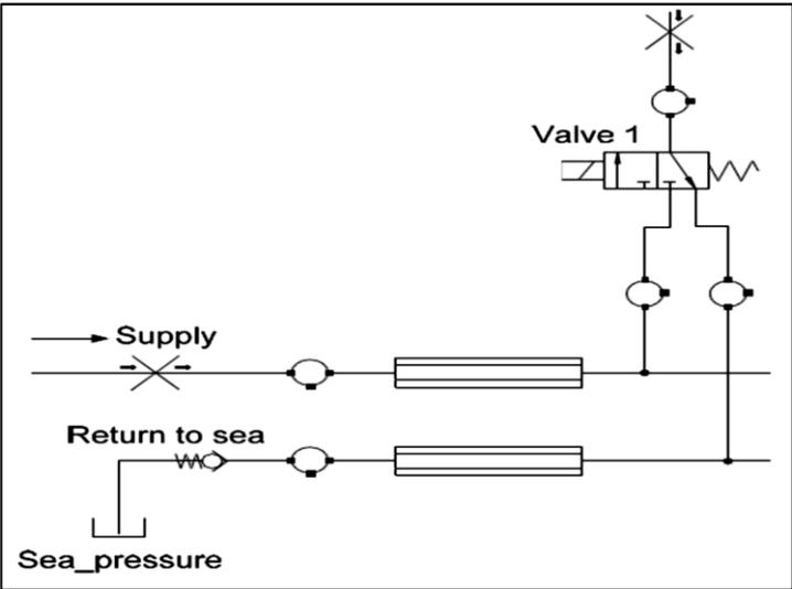
Figure 19. Subsea Control Module model [7]
