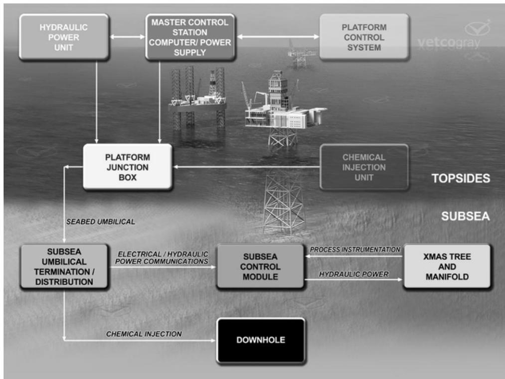
Figure 2. Subsea Control Module Schematic [5]
