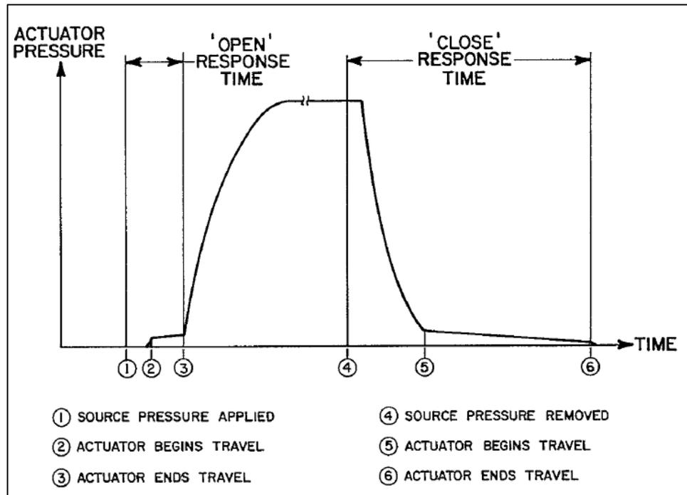
Figure 8. Typical response curve with stainless steel control line [13]
