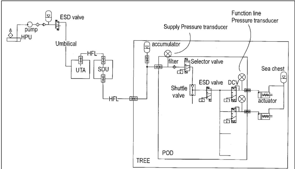
Figure 9. An embodiment of an overall hydraulic control system for a subsea project [15]
