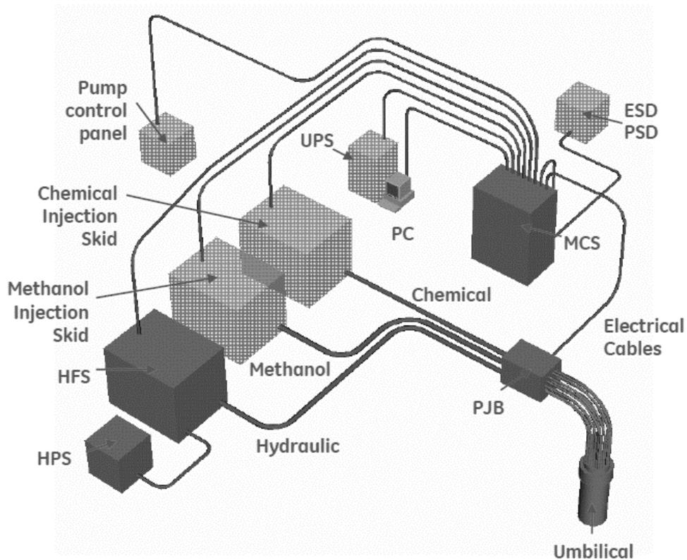
Figure 3. Top side control equipment [5]
