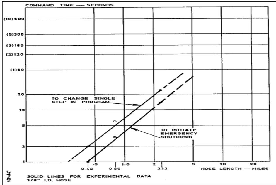
Figure 7. Hydraplex mode delay time vs hose length [11]
