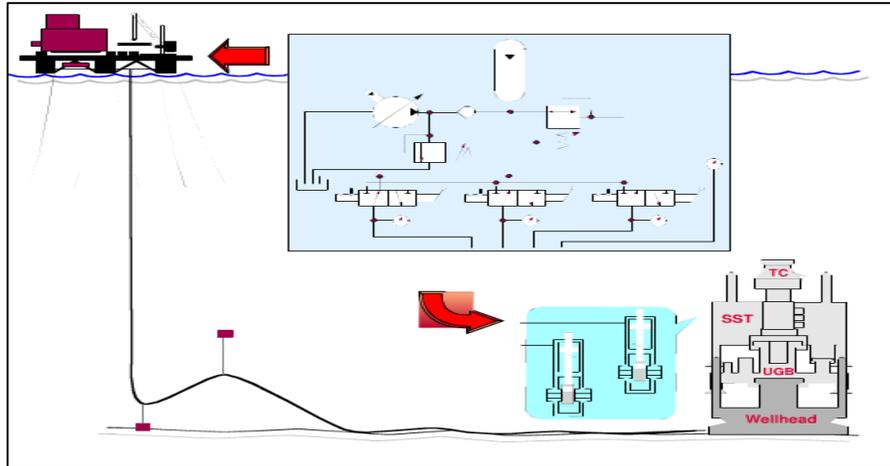
Figure 6. Direct Hydraulic Control System [9]
