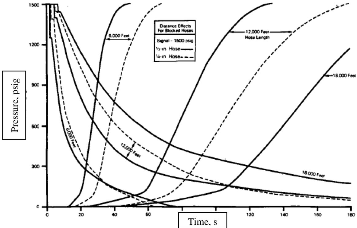
Figure 39. Effect of hose size and length on signal response from Cadlao [19]
