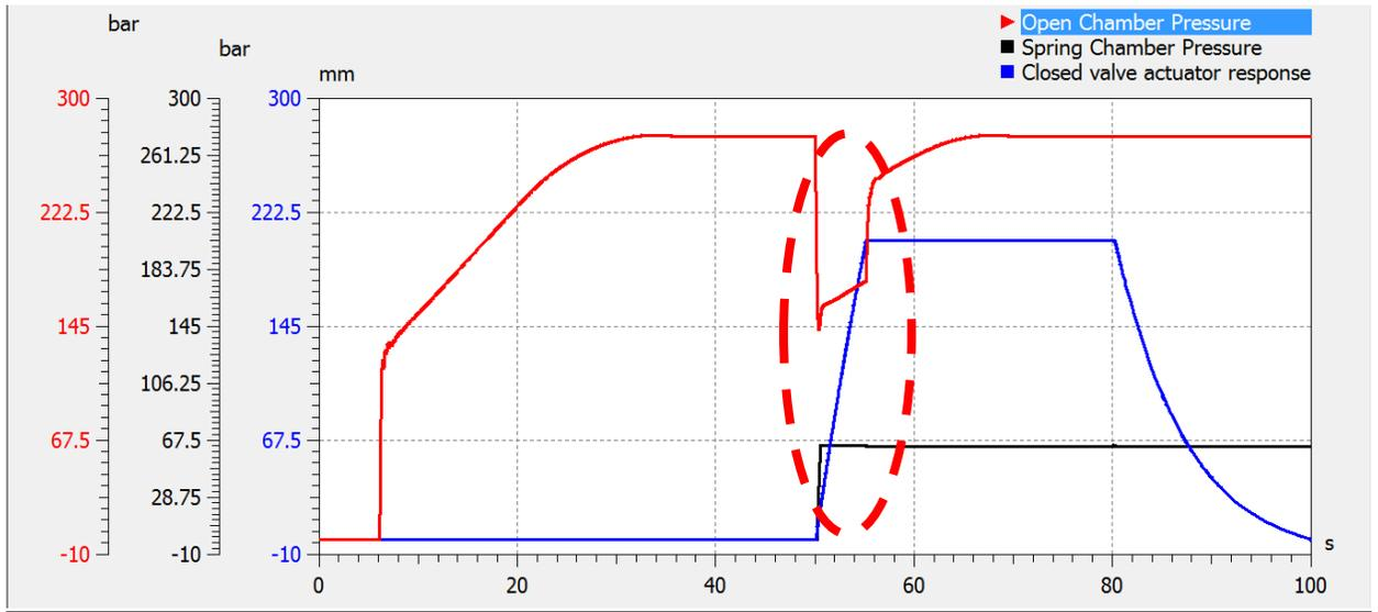
Figure 34. Pressure response curves for the open gate valve #2
