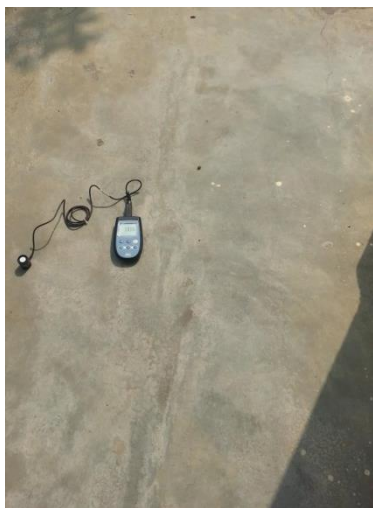
Figure 25 Illuminance Measurement in Unshaded Area
