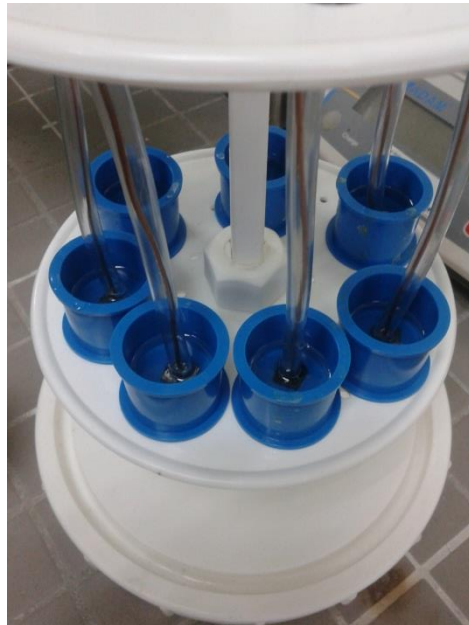
Figure 3.5: Moulded samples inside cylinder-shape rings
