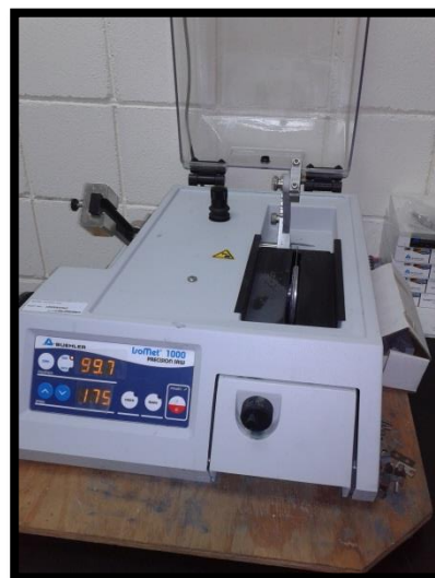
Figure 3.2: Precision saw machine for sectioning purpose
