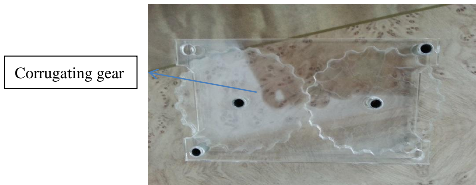
Figure 16: Sample of corrugating gear
