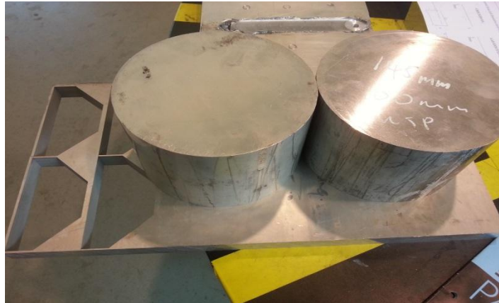
Figure 24: Work piece before cutting using EDM wire cut
