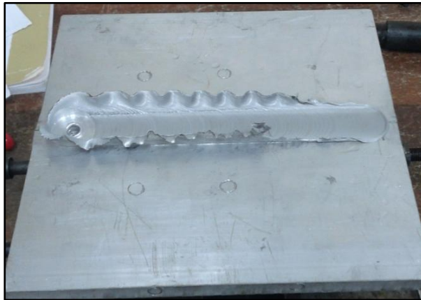
Figure 10: The sample of the FSP trial (Al-6061)
