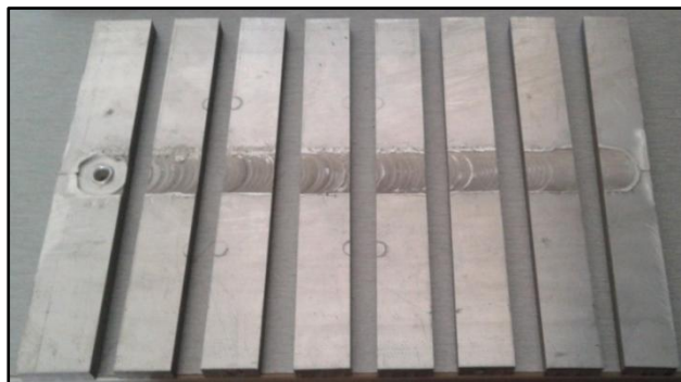
Figure 11: The FSP samples after cut by EDM Wire-Cut
