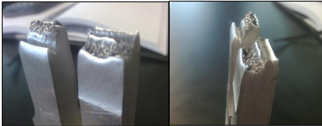
Figure 12: Fracture at one of the sample tested
