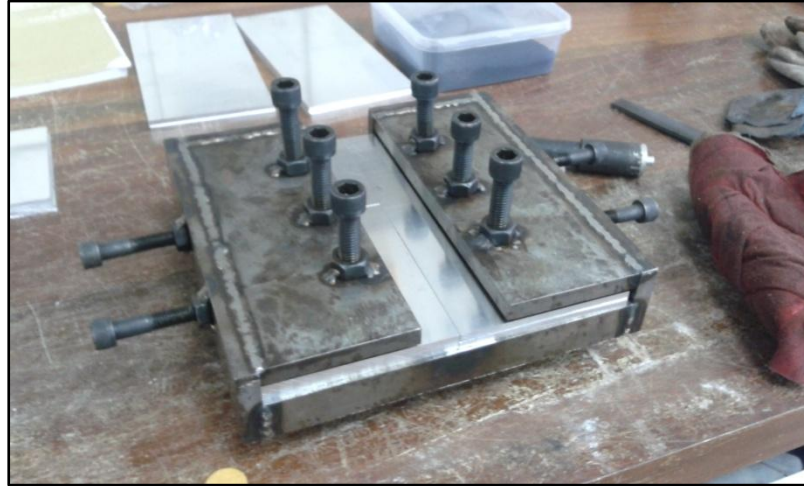
Figure 4: The Aluminium plates placed inside the jig
