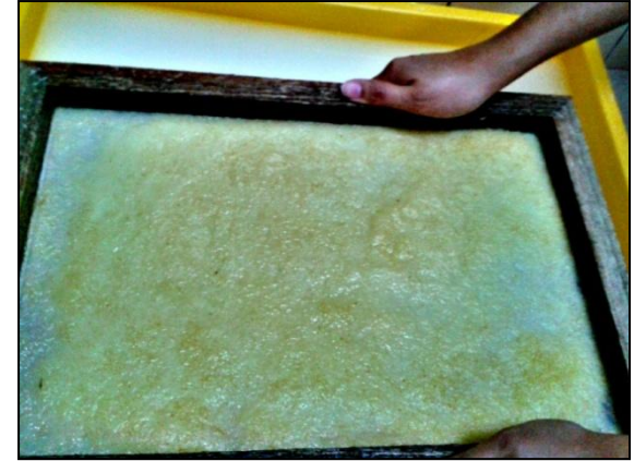
15. Filtration of the pulp on the silk screen.
