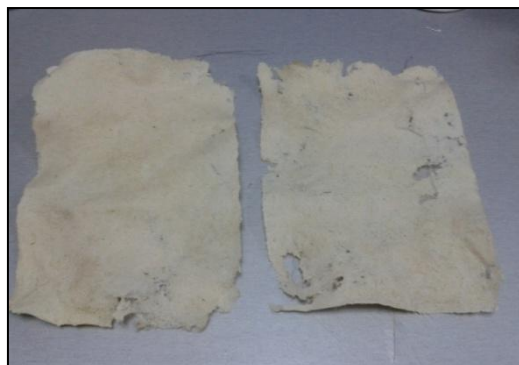
FIGURE 13: Two sheets of paper produced from 100g bagasse.
