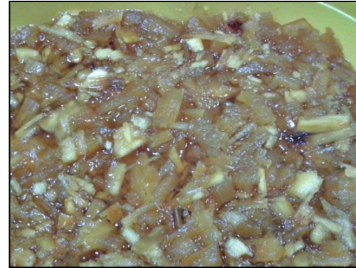
10. Bagasse is soaked in 10% sodium hydroxide solution.
