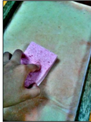
17. Drying up of the filtered residue with sponge
