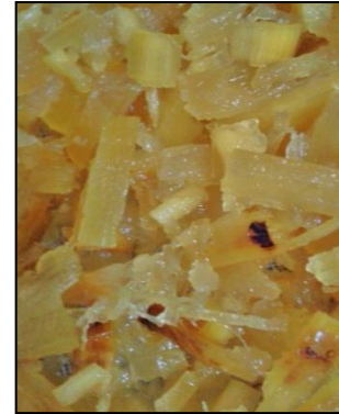
10. Bagasse is soaked in 10% sodium hydroxide solution.
