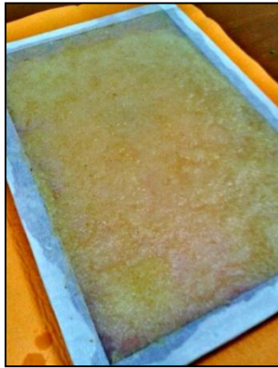
16. Filtration of the pulp on the silk screen.
