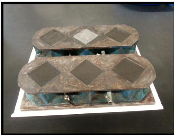
**Figure 34:** Cement slurry of Composition 1 in the moulds.
