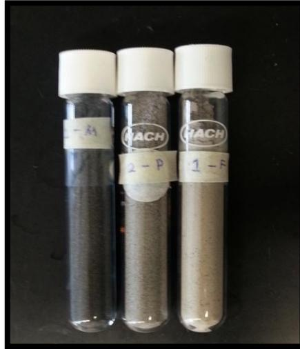
**Figure 37:** Samples of MIRHA, FA and POFA for FTIR.
