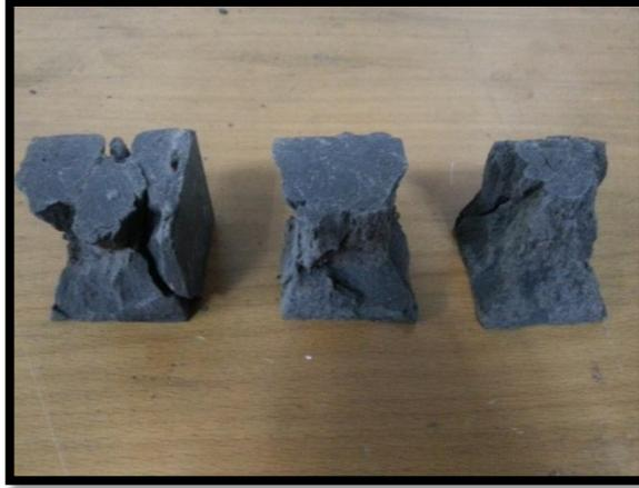
**Figure 44:** Crushed cement cubes of 7 days curing of Composition 2.
