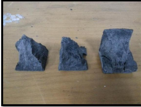
**Figure 48:** Crushed cement cubes of 14 days curing of Composition 1.
