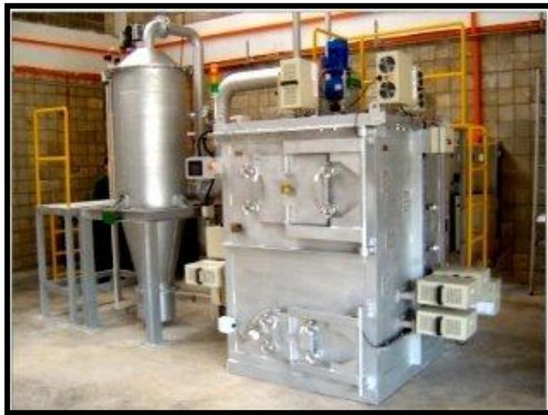
**Figure 5:** Microwave incinerator (Vishie, 2009)
