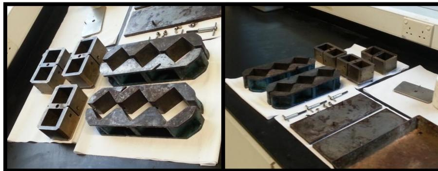
**Figure 33:** Cement Moulds
