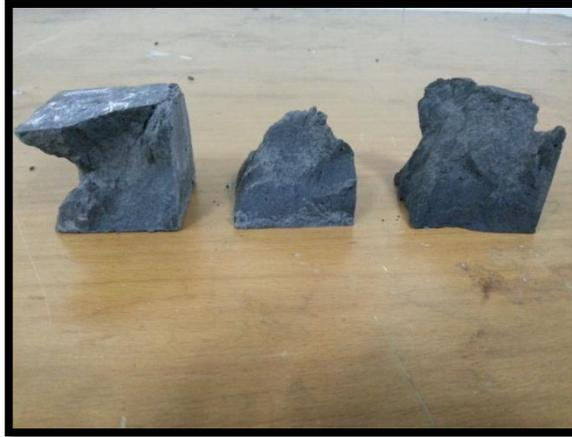
**Figure 40:** Crushed cement cubes of 7 days curing of Composition 1.
