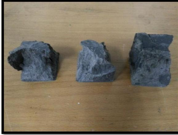
**Figure 52:** Crushed cement cubes of 14 days curing of Composition 2.
