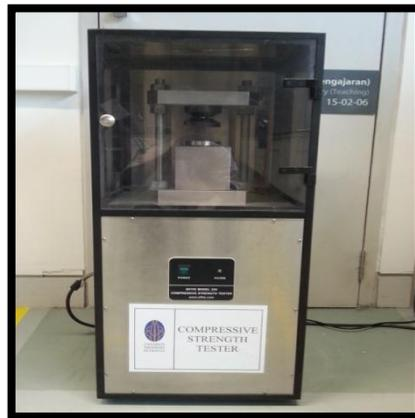
**Figure 31:** Compressive Strength Tester
